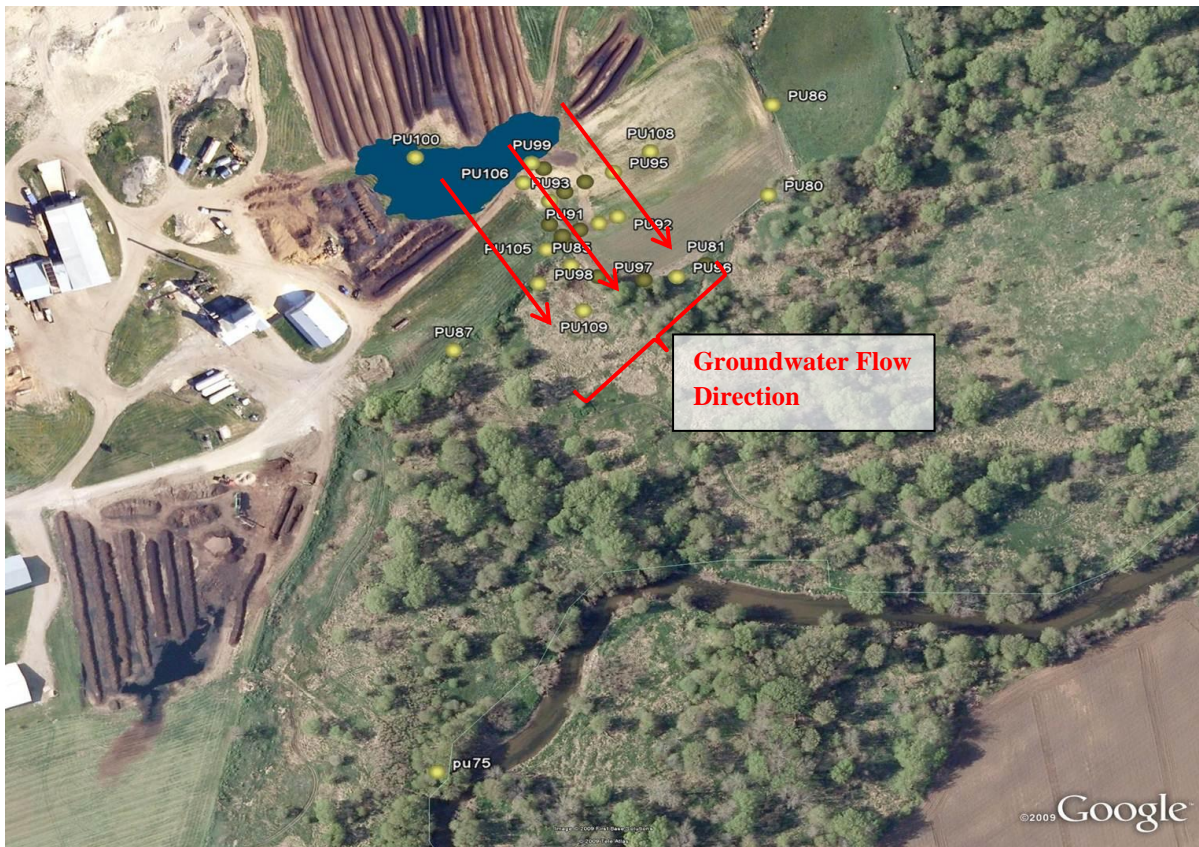
Figure 4: The Putnam Turkey manure site seen by satellite imaging. The numbers refer to the well location.
