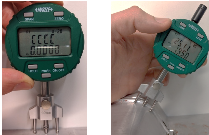
Figure 4-3: Zeroing radius gauge (left) and radius measurement (right)
