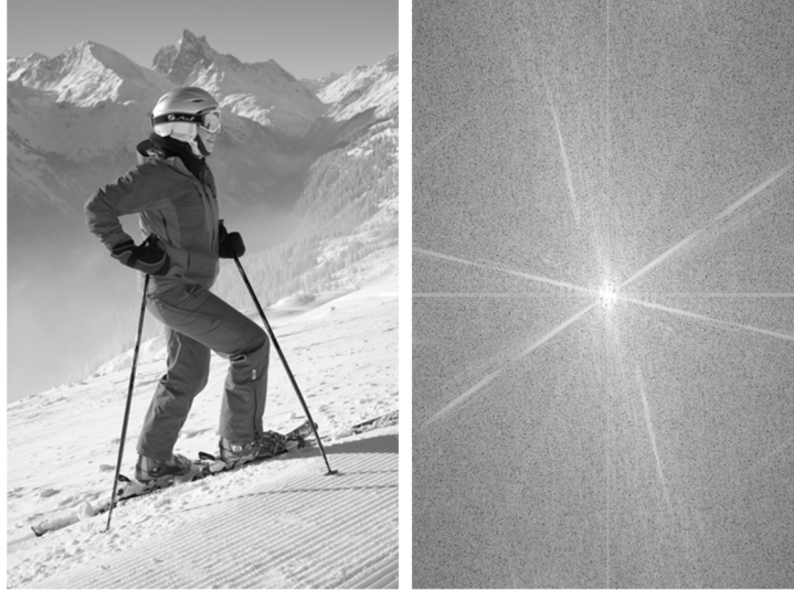
Figure 2-7: Image transferred into frequency domain. Left: spatial domain. Right: frequency domain.
