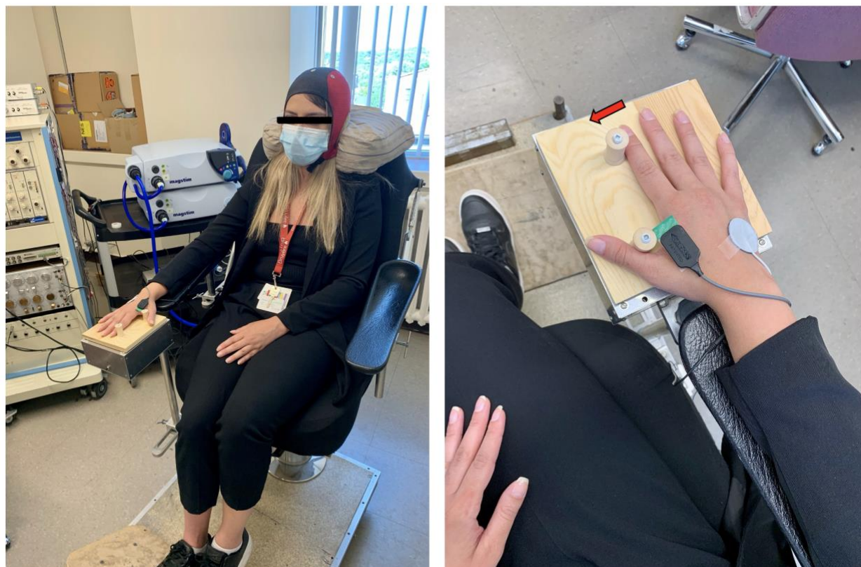
Figure 3.2 Experimental setup including the apparatus used to delimit the index and thumb finger position (right). Activation of FDI is achieved by pressing the index finger lightly against the top block.
