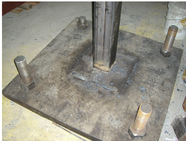
Figure 2.7-Column-Base Plate-Strong Floor Connection
