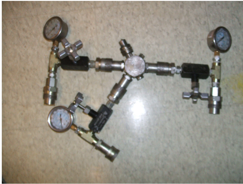
Figure 2.11-System of Needle Valve Couplers
