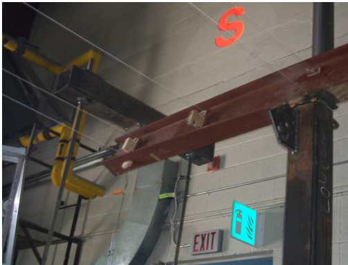
(c) Buckling Configuration Specimen 2 (Buckling Load = 54.3kN)
