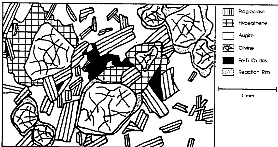
Figure 4.18. Thin section sketch illustrating reaction rims and hypersthene coronas on olivine in ophitic olivine-hypersthene gabbro in the central regions of sill C. Sample F90-80.
