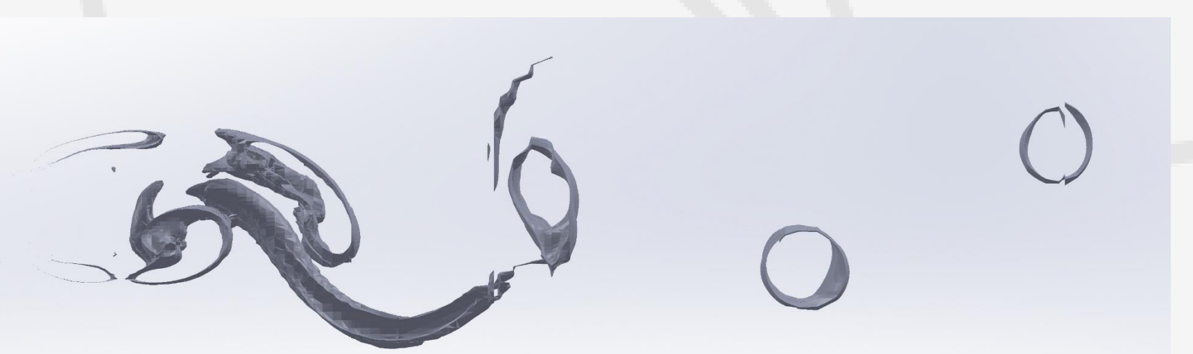
Figure 1. Two-dimensional view of flow past a square cylinder exhibiting vortex shedding
