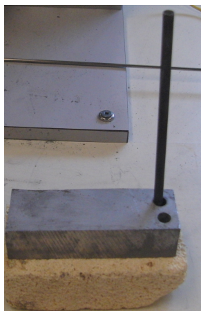
Figure 4.20: Filled tube and the holder before ignition
