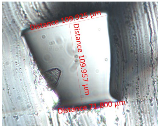
Figure 16 Dimensions of the first test of fabricating wafers using photolithography: Left (top width: 110, bottom width: 72, height: 110) right (top width: 114, bottom width: 59, height: 104)
