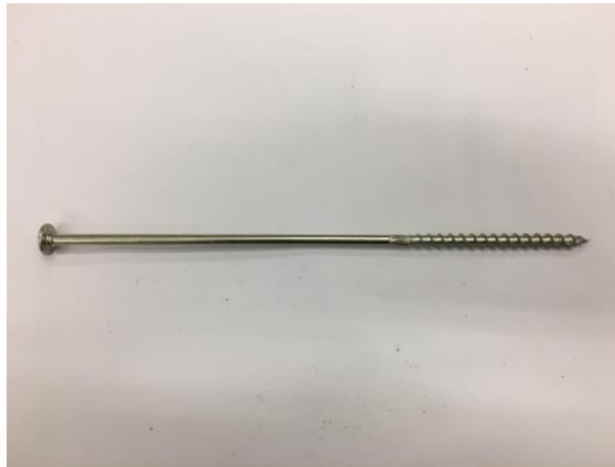
Figure 3.5: Screw D – 8x300 Heco-Topix Zn Gelb A2L
