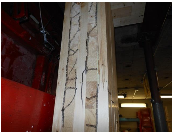
A) Left Side Flexural Failure
