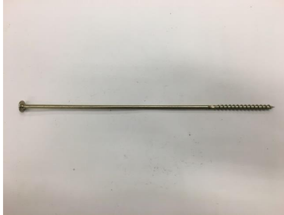
Figure 3.4: Screw C – 6x300 Heco-Topix Zn Gelb A2L
