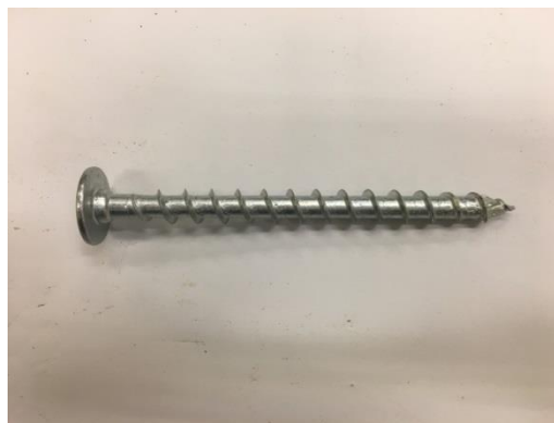
Figure 3.3: Screw B – 10x120 Heco-Topix Zn Blau A2K
