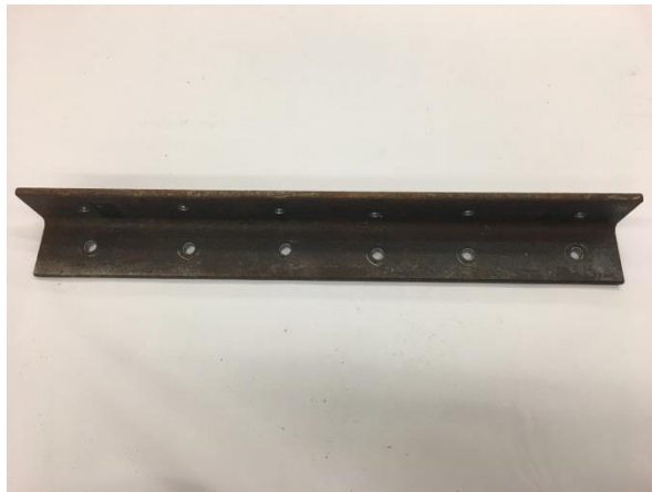
Figure 3.8: Angle B – Stiff Manufactured Angle
