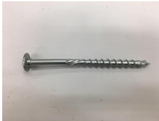
Figure 3.2: Screw A – 8x120 Heco-Topix Zn Blau
