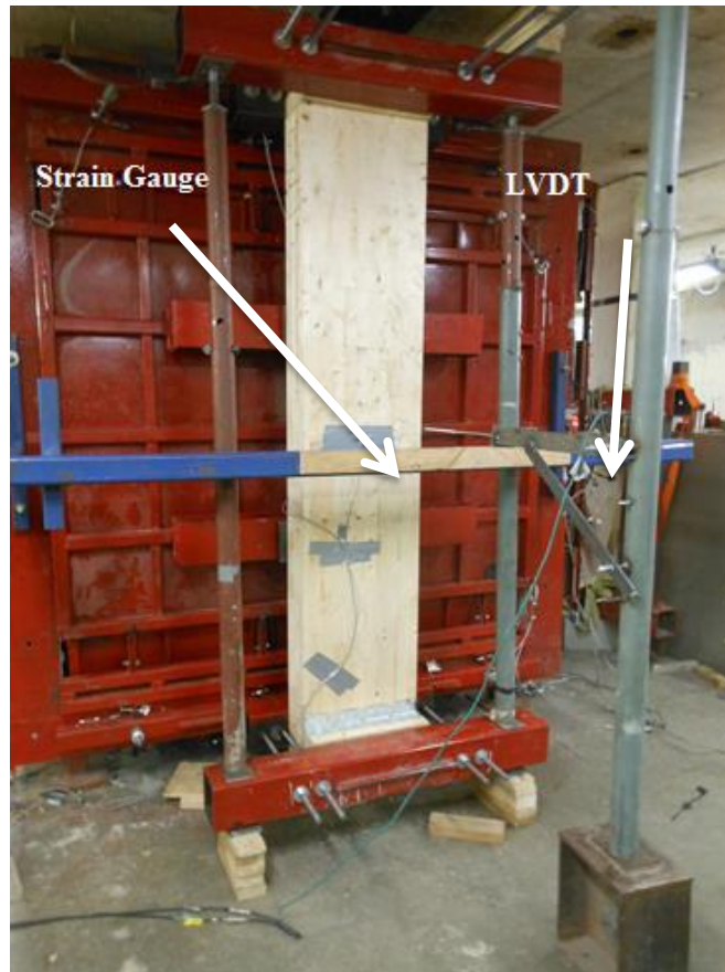
Figure 3.18: Measurement Device Placement
