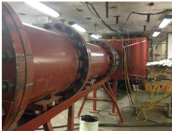
Figure 3.11: Shocktube Driver and Diaphragm Section
