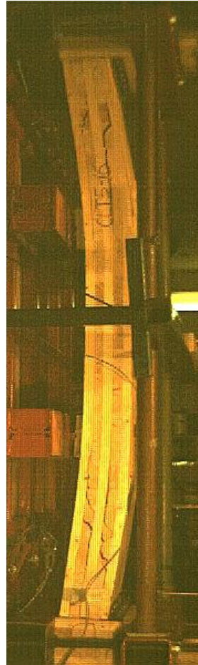
Figure 5.7: CLT5-10 at Maximum Displacement (85 mm at 41ms)
