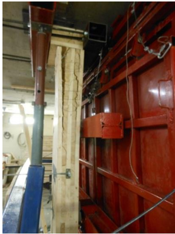
A) Perpendicular to Grain Failure
