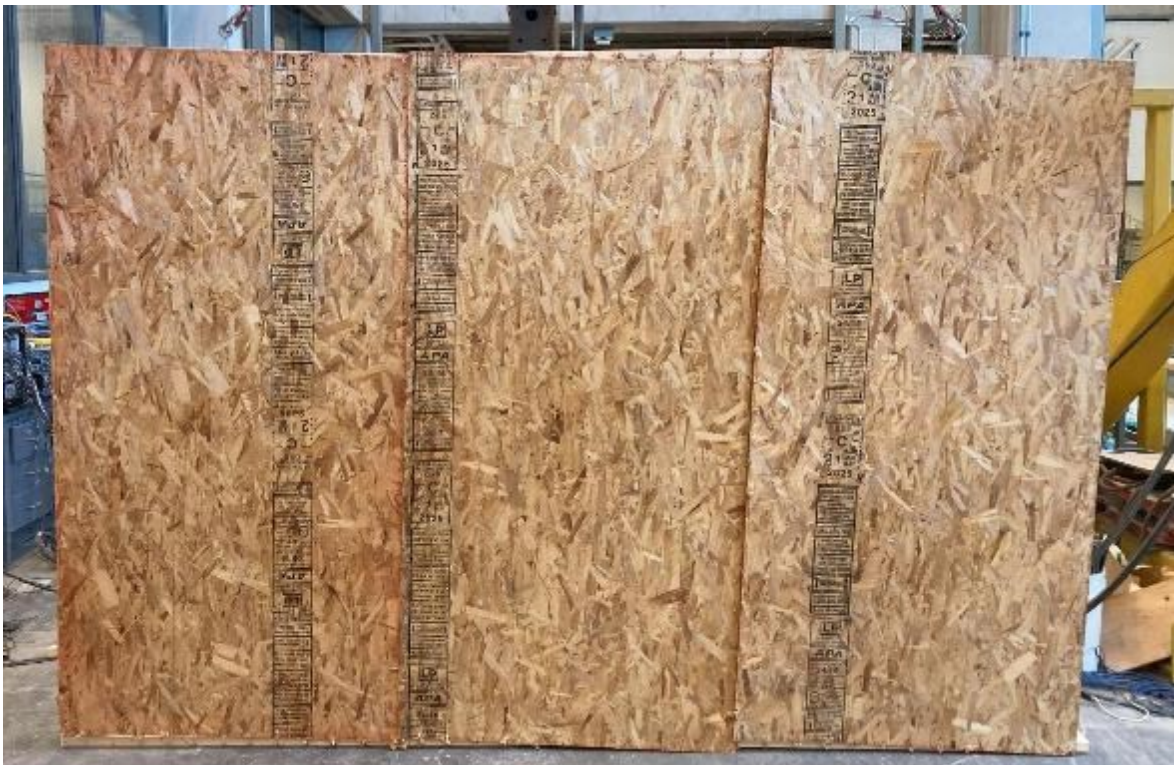
Figure 4.56: Shear wall Configuration #12 (after test)
