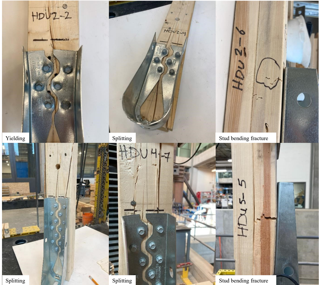
Figure 4.19: HD failure modes
