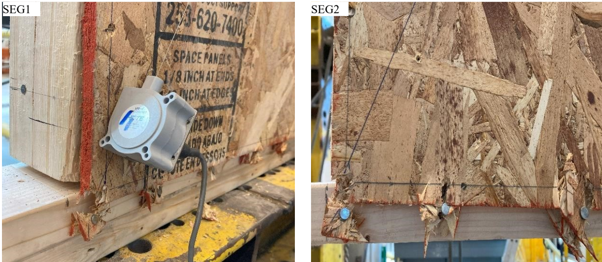
Figure 4.36: Sheathing panel tearing and nail failures in Configurations #3
