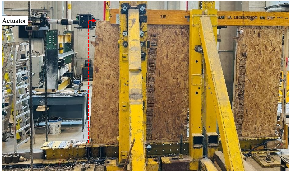
Figure 4.25: Shear wall test setup in Configuration #1
