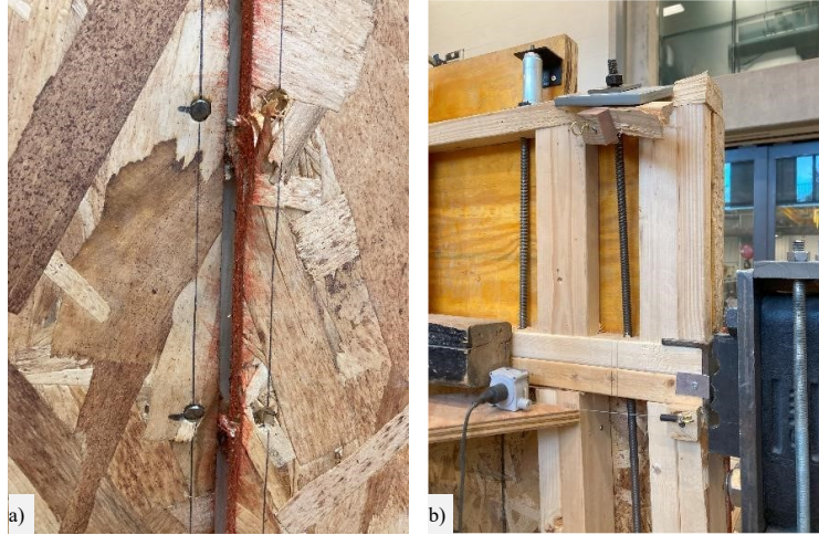
Figure 4.58: (a) nail failure at panel interface; (b) failure of the ATS rod system
