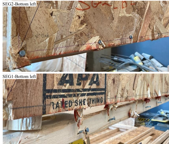
Figure 4.44: Nail failures at the bottom edge of shear walls in Configuration #5
