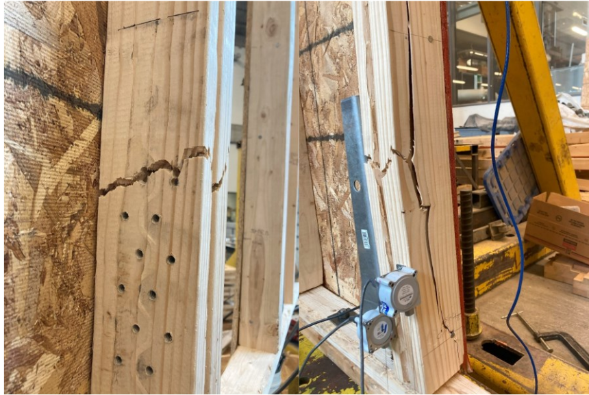
Figure 4.50: SEG2 tension chord fracture in Configuration #8
