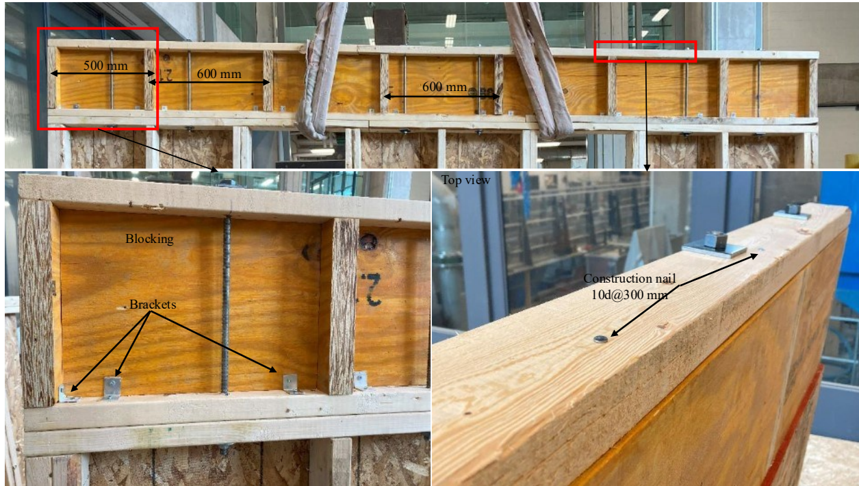
Figure 3.14: Blocking floor assembly configuration
