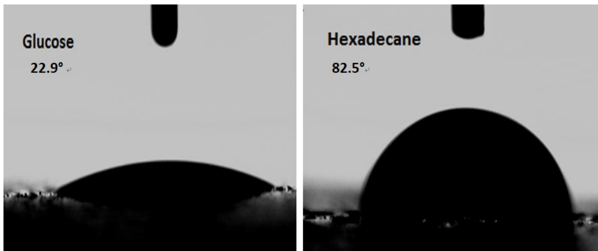
Figure 4.20 Changes in contact angle of R. erythropolis EPWF after 8 d growth in BHMV medium with 50 g/L NaCl and either glucose or hexadecane as the carbon source.
