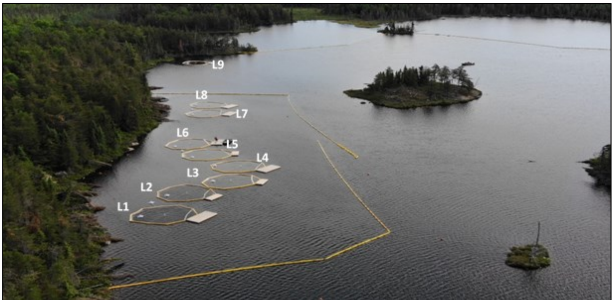
Figure 2.3: Overview of the nine limnocorrals used for the simulated dilbit spill conducted at Lake 260.
