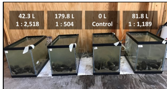
Figure 2.4: Aquaria used to house the giant floater mussels. The amount of dilbit added to the respective limnocorral and resulting dilbit:water dilutions of each aquarium are labelled on top.
