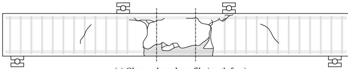
(a) Observed crack profile (north face)
