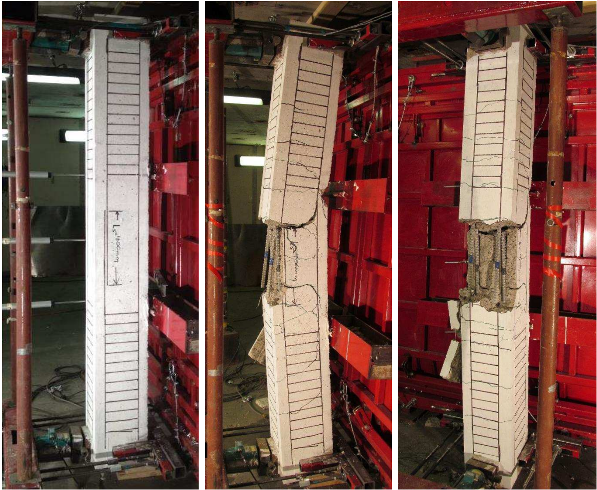
(a) Before high strain rate testing (b) After high strain rate testing (c) After high strain rate testing
