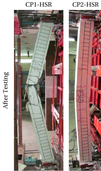
Figure 4.15: Comparison of splice damage for beams with 10M reinforcement.
