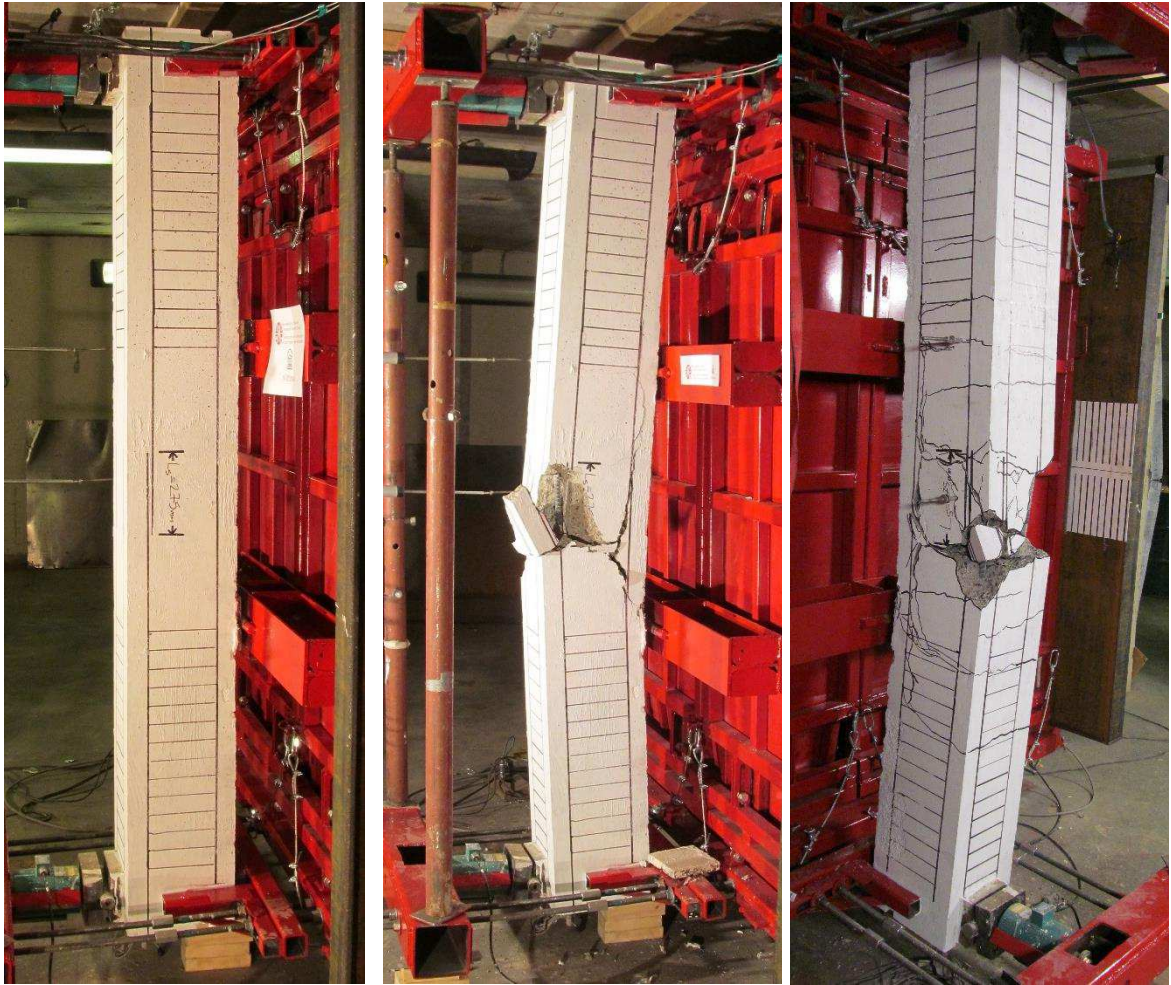
(a) Before high strain rate testing (b) After high strain rate testing (c) After high strain rate testing
