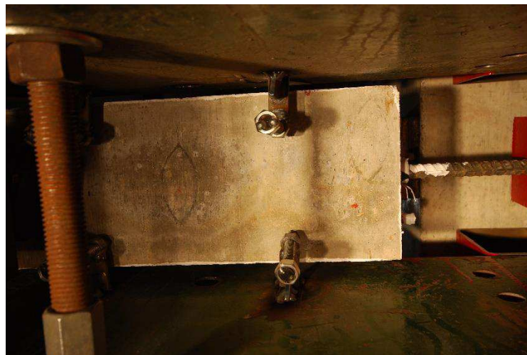
Figure A.7.2.1: Photograph of the underside of BE7 after Test 2.
