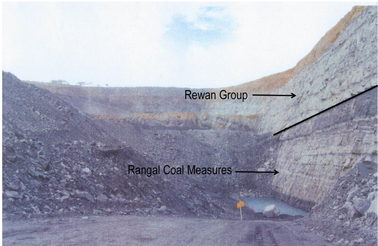
Figure 11: Contact between the Rangal Coal Measures and the Rewan Group in the Burton Mine highwall located immediately to the east of the New Lenton deposit area.
