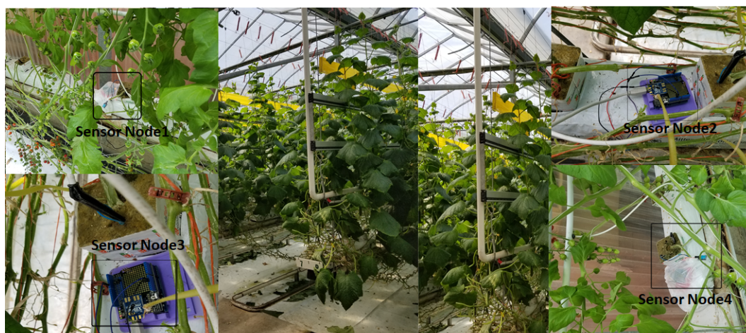
FIGURE 8.1: A snapshot of how sensor nodes are deployed in a greenhouse (only few nodes are shown)
