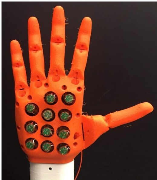
Figure 6.1 Prototype of an Ada robot hand with palm embedded multi-modal bio-inspired tactile sensors
