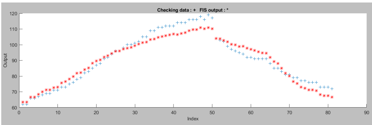
Figure 5.43 Actual vs ANFIS output for the ring and pinky fingers
