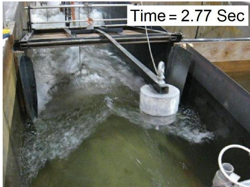
Figure 6.2. Cross-waves occurring upstream of the column in the physical experiments (experiment E-85-C).
