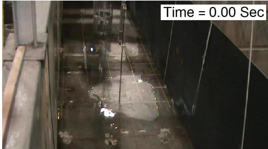
Figure 4.4. Partially dry-bed condition observed in some of the experimental runs.
