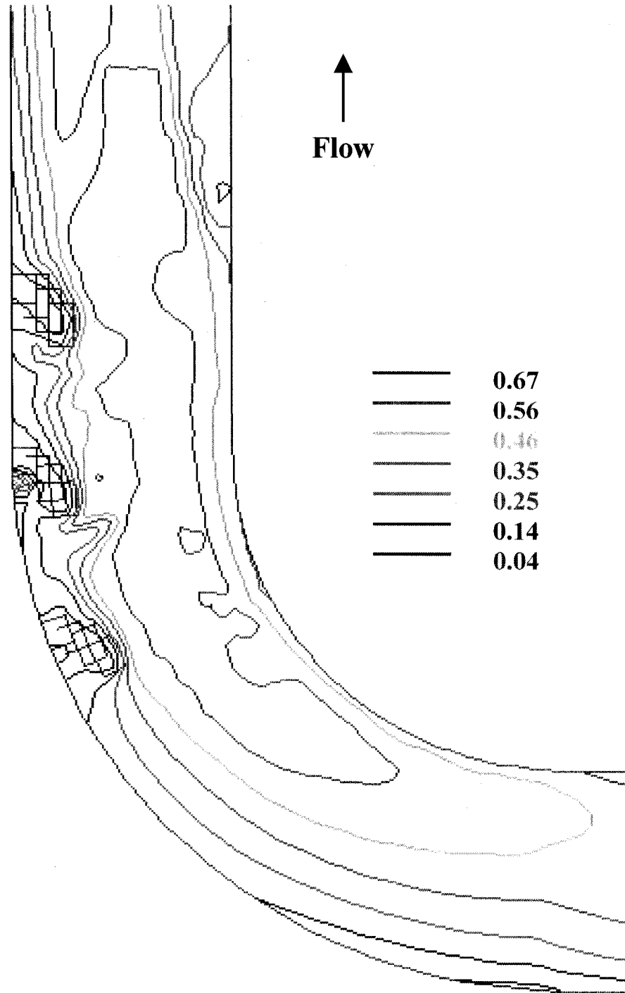
Figure B.18 Predicted bed shear stress distribution: 90° bend, Group B, \theta = 40^\circ (in \text{N/m}^2 ). Channel wall and blocked out regions (barbs) in red.
