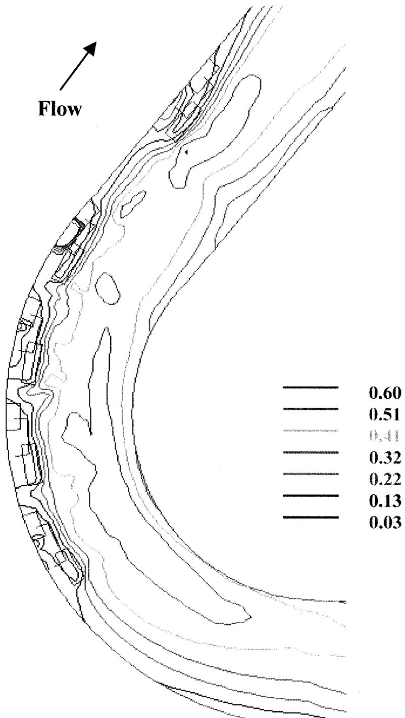
Figure C.6 Predicted bed shear stress distribution: 135° bend, Group B, \theta = 20^\circ (N/m 2 ). Channel wall and blocked out regions (barbs) in red.
