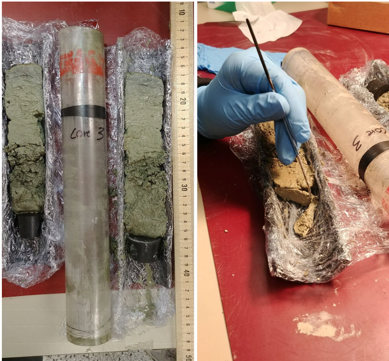
Figure 3–4 Split Core 3 prior to sampling (left), and sampling of the microbial mat laminae (right) at the Department of Geography laboratory facilities at the University of Ottawa.
