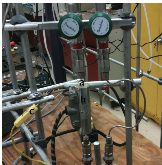
Figure 7 Microreactor setup showing alumina tube (a) as reaction chamber surrounded by a furnace (b) and thermocouple (c).
