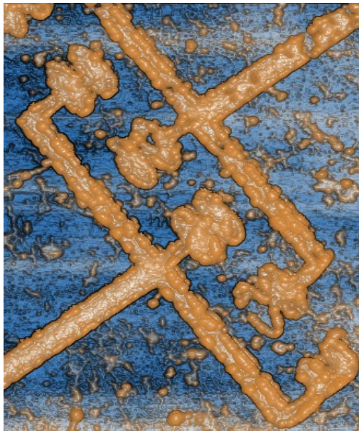
Figure 58: AFM for the electrode with DEP parameters 2 V_{pp} , 150 kHz and 3 secs
