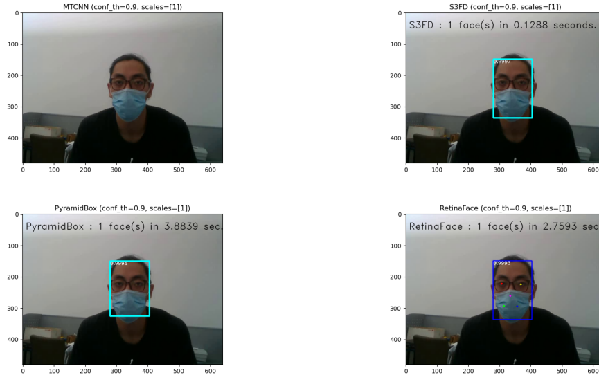
Figure 4.12: Face detection results using different face detectors.
