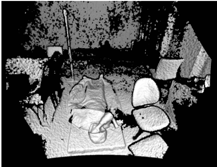
Figure 1.3: Example of a subject lying covered with a blanket where Microsoft Kinect system was not able to detect the subject.
