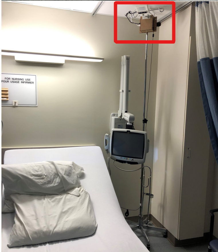
Figure 3.1: The depth-radar monitoring system.
