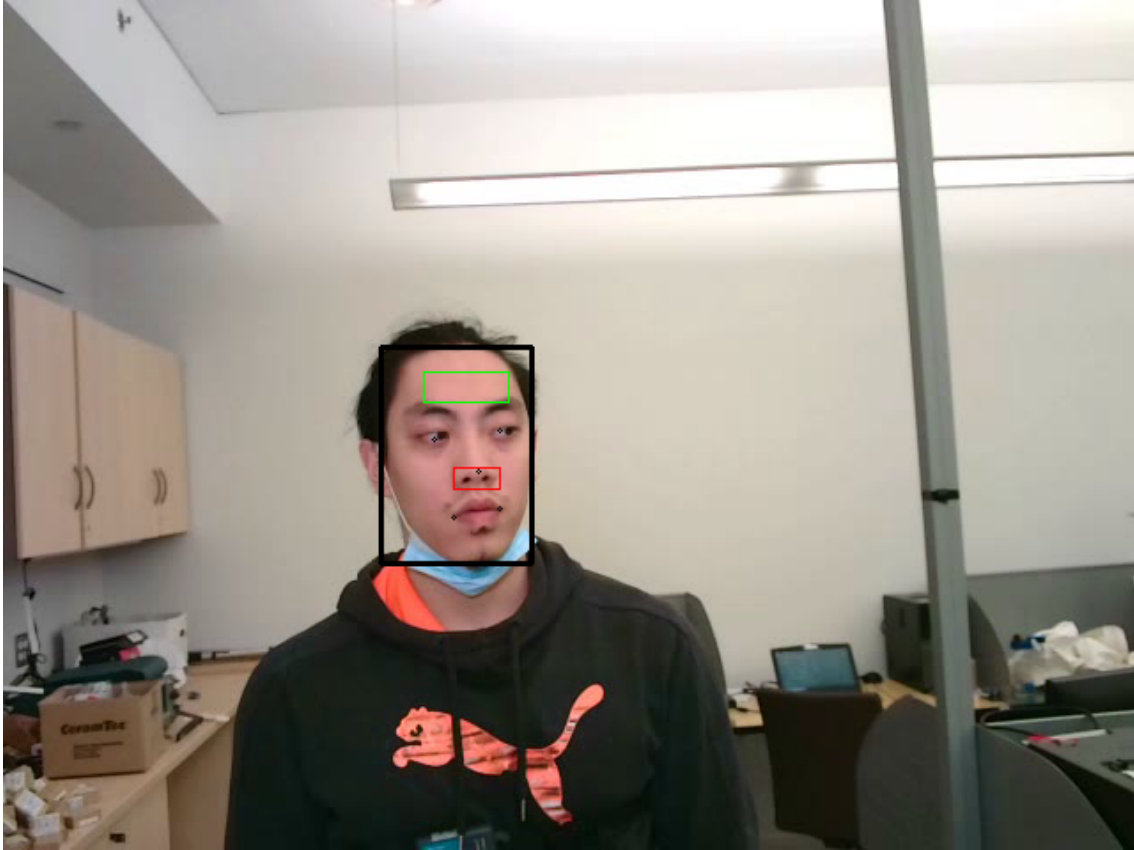
Figure 3.11: Facial landmarks and partitions detected at 1.2m.
