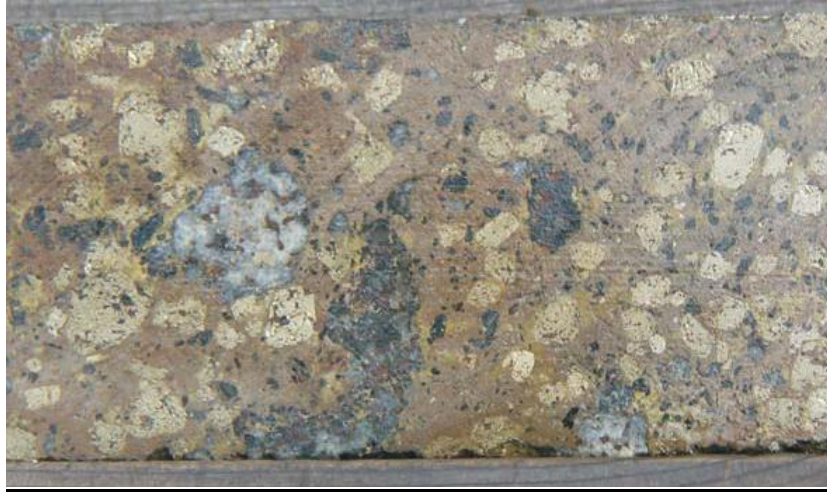
Figure 7: Photograph of classic durchbewegung texture (Craig and Simpson, 1991) in type 1 Fe-Zn-rich massive sulfide ore (DUB195, 809.7 m). The texture shows rounded nodule of hard pyrite and quartz in a matrix of softer sphalerite. NQ drill core (47.6 mm or 1-7/8 in diameter).
