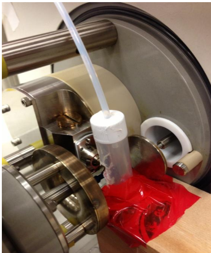
Figure 8: QTOF2 setup to attempt protonating using acid spray. Here is shown an attempted setup to build up acidity in gas form.
