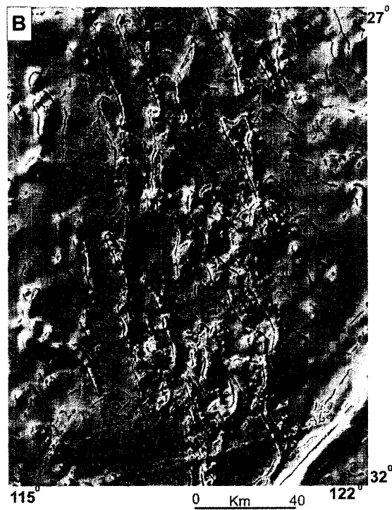
Figure 3.4: Earthworms calculated for the studied areas ; A: Pilbara craton. B: Southern Cross granite-greenstone Terrane. C : Abitibi Subprovince. The dots correspond to the maxima of the horizontal gradients calculated for each surface, from red (10 km upward continued) through yellow (5 km) to blue (Earth's surface).
