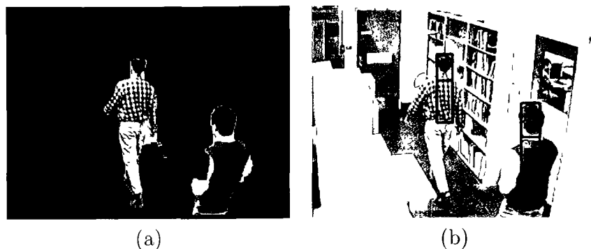
Figure 5.1: (a) Segmented image of two people. (b) Image showing two people with the region in which the percentage of pixels is computed to determine if a person is detected
