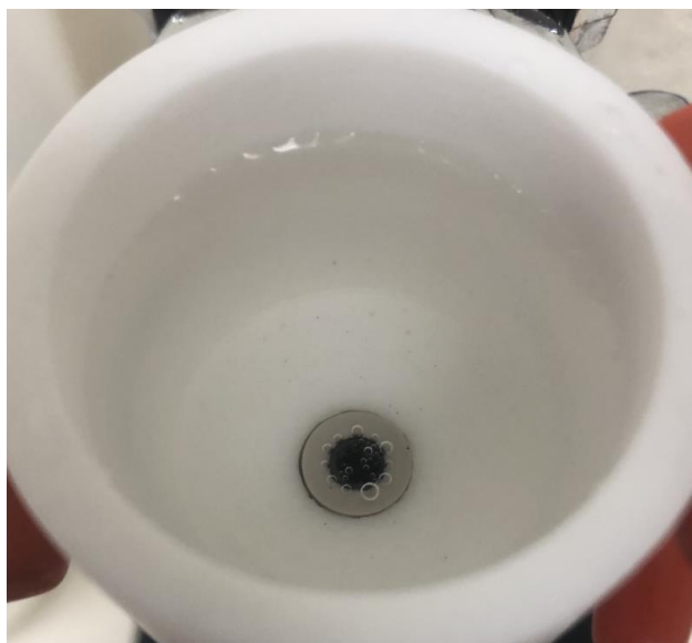
Figure F.4: The Ni_{90}Fe_{10} electrode with 42 wt% Nafion TM post-OER testing using Method 2 of working electrode preparation.
