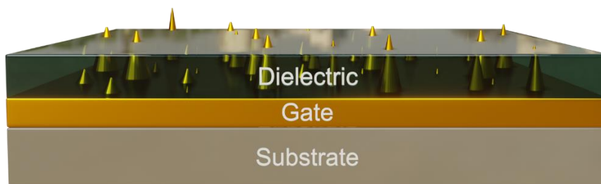
Figure 1.8. Example of pinholes caused by the surface roughness of the metal electrodes and how they can cause short circuits.
