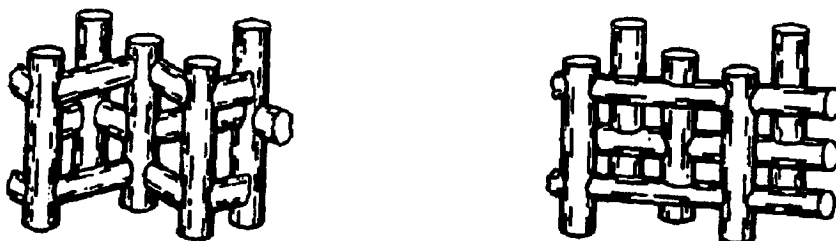
Figure 1.4 Alternate depiction of the channel structure of zeolites ZSM-5 (right) and ZSM-11 (left). (Reproduced with permission from reference 27).
