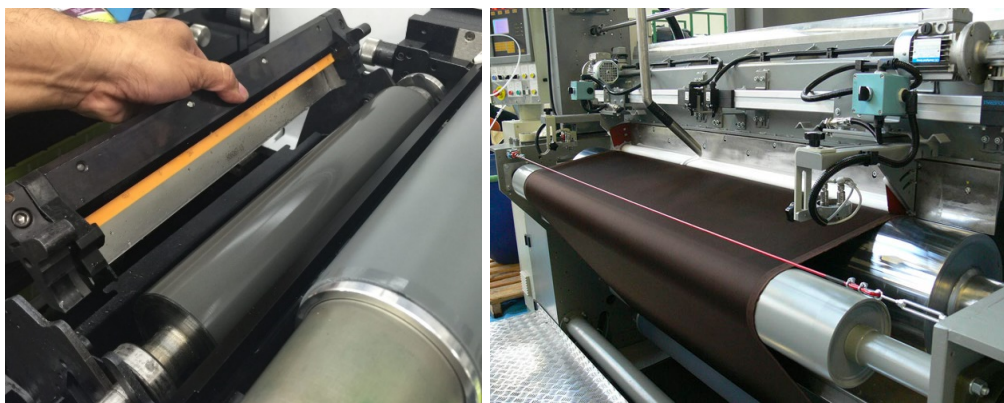
Figure 1-2: Roll-to-roll blade coating [57, 58].
