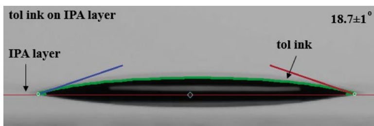
Figure 3-18: Contact angle of a TOL-based reducer ink drop on a blade coated IPA based precursor layer.
