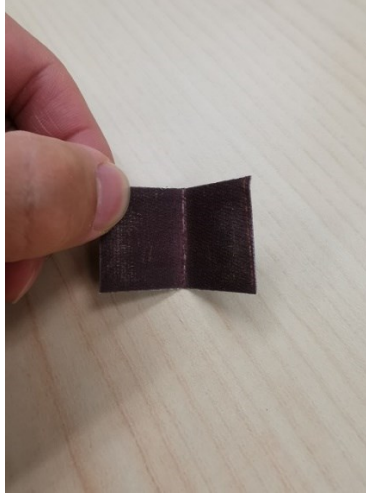
Figure 3.47 Kapton insulation removal tool made by sandpaper piece.
