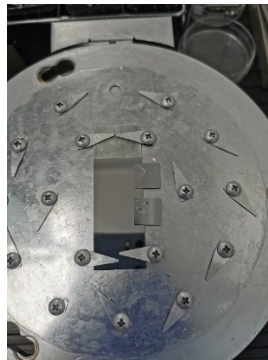
Figure 3.41 Sample glass side mounted on the evaporator sample holder.
