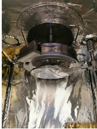
Figure 3.42 Assembled sample holder with the shutter closed.
