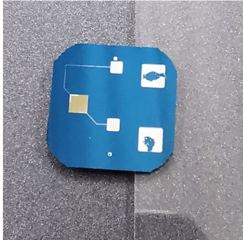
Figure 3.50 Adhesion issue between aluminum layer and SiN layer.
