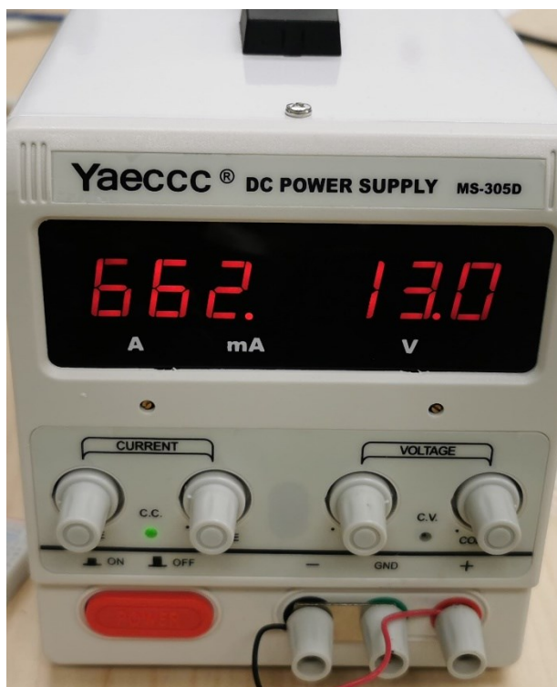
Figure B7 The power supply for the pad heater to melt the crystal bond piece. The current and the voltage should be set as shown in the picture for melting the crystal bond.
