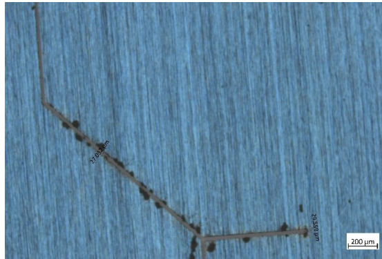
Figure B3 Image of shadow mask feature machined by laser under the microscope.
