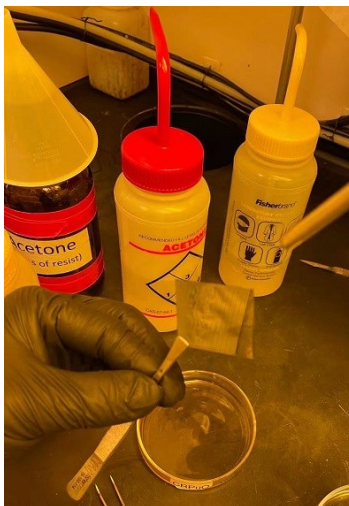
Figure 3.10 Blowing Method for Drying Membranes with N 2 Gun
