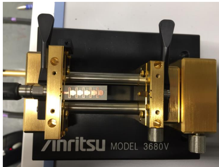
Figure 37 Antenna measured with Anritsu 3680V test fixture
