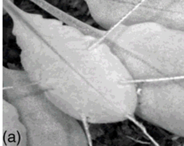
Figure 1.5: Experimental set-up digital image sequence analysis method. The leaf is pulled into a flat position by weights threaded through its margins. From Wiese et al., 2007.
