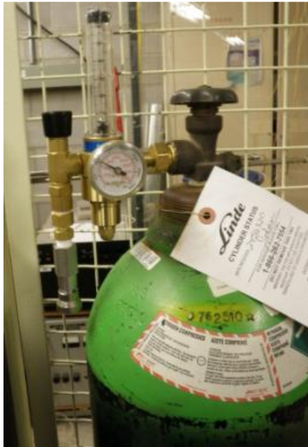
Figure 42. Feeder Gas Bottle. Gas From This Bottle is Fed into the Powder Feeder
