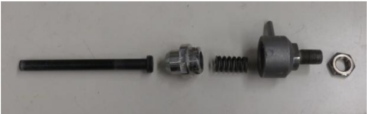
Figure 145. Disassembled de Laval Plastic Nozzle Showing, From Left to Right, Plastic Nozzle, Quick-Connect Cap, Spring, Orifice and Heater Nut
