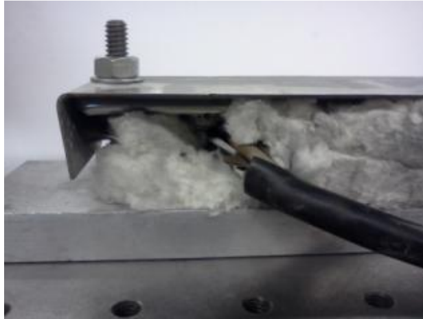
Figure 108. Side View of the Heater Assembly, Showing the Heater underneath the Steel Barrier
