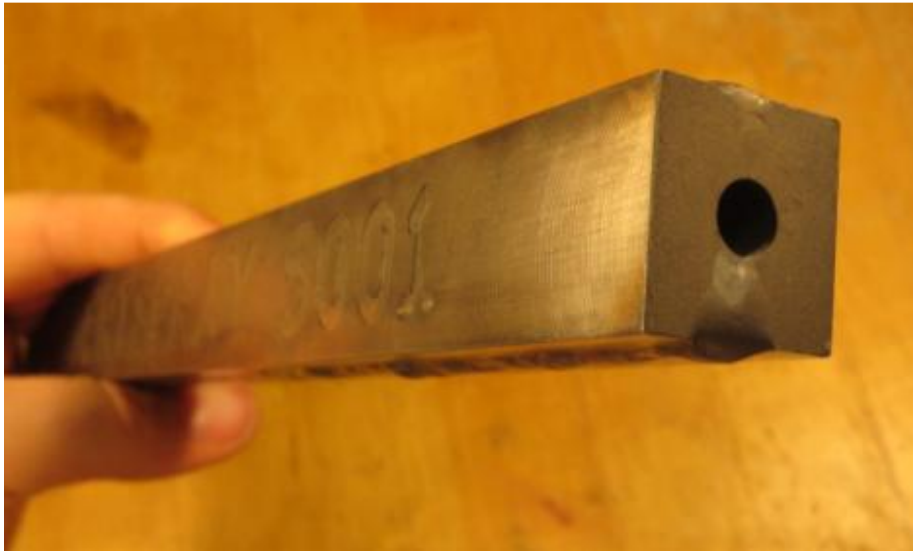
Figure 150. PR Nozzle, View of the Exit Area
