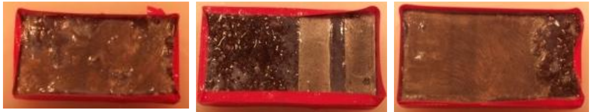
Figure 92. ASTM G34 As-FSW Samples (a) Ground Substrate (b) As-Received Substrate (c) Ground Substrate
