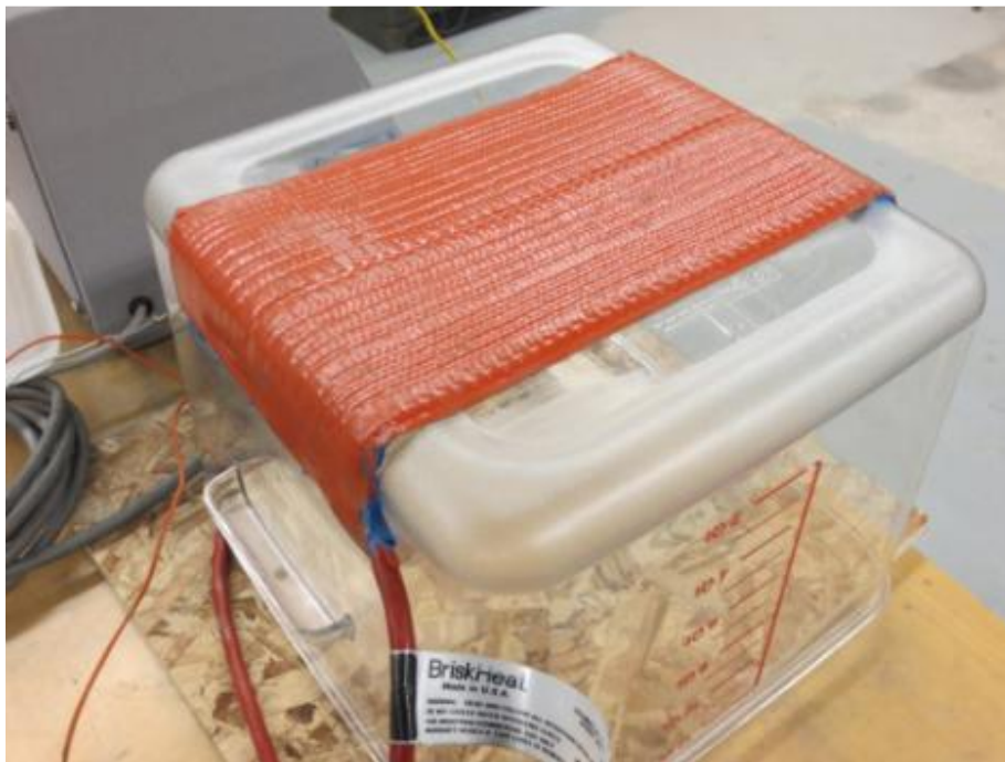
Figure 59. Corrosion Test Apparatus Glued Heated Pad
