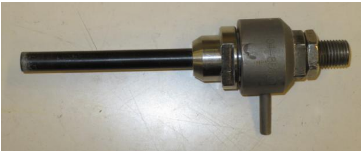
Figure 146. Assembled de Laval Plastic Nozzle Assembly
