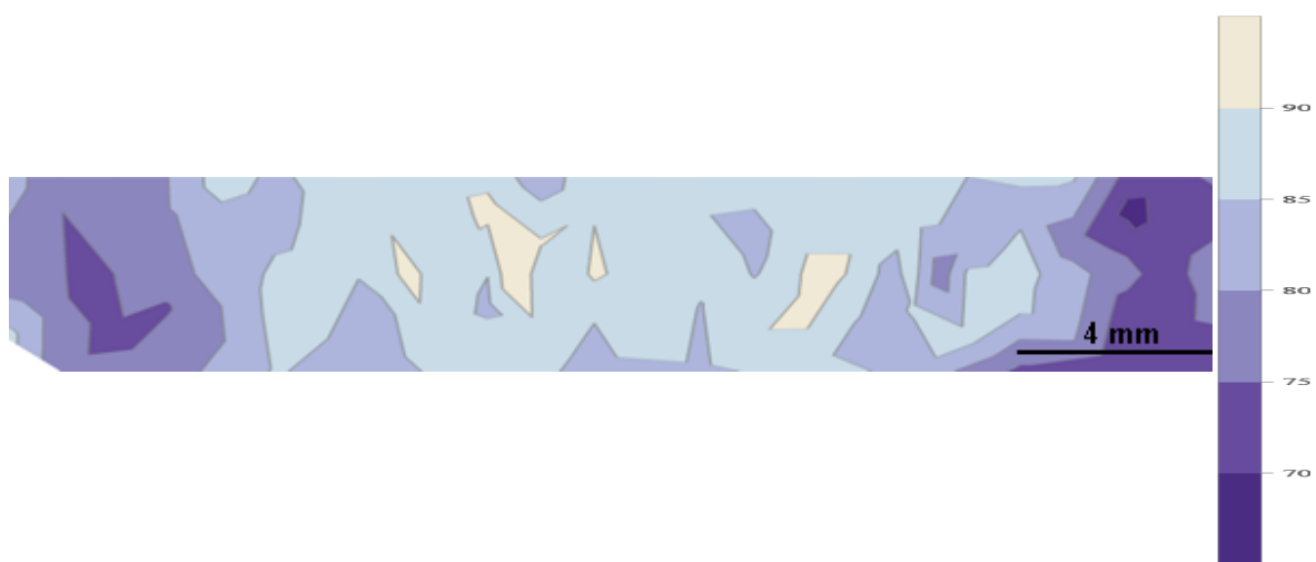
Figure 78. 4 mm Al 6061 FSW Hardness Mathematica Contour Plot. (110 Indents) Scale Indicates Vickers Hardness. Weld Regions are Represented by the Following Hardness Ranges: Weld Nugget 85-90 Hv, TMAZ 80 Hv, HAZ 70-75 HV
