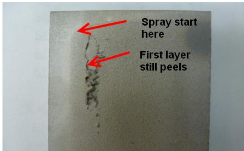
Figure 125. AA 7075 Spray Started on the Substrate to Eliminate Potential Edge Effects
