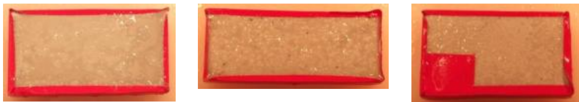
Figure 94. ASTM G34 Al 5083 Samples (a) Ground Substrate (b) As-Received Substrate (c) Ground Substrate
