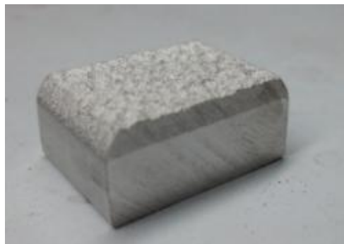
Figure 46. Typical Example of Sample After Cutting Process. Note the Aluminum Coating on Top (Pure Al) and the Saw Marks on the Cut Side (Facing Front). Sample is 3/8" wide
