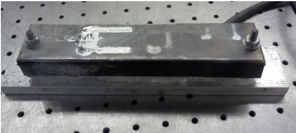
Figure 109. General View of the Heater Assembly
