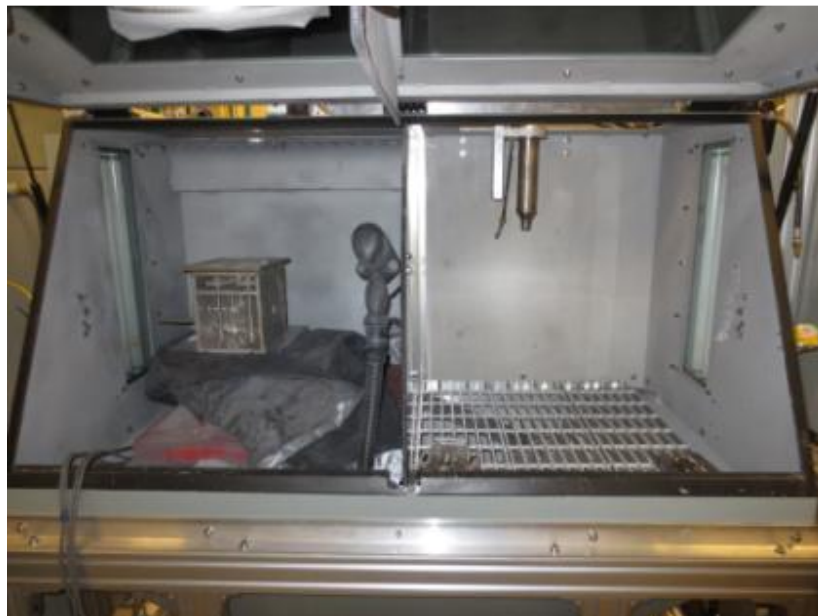
Figure 37. Open Cabinet Assembly. Right Half Contains the CGDS System Spray Booth
