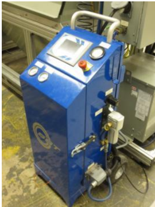
Figure 39. Pressure and Temperature Controller Feed Propellant gas to the Heater
