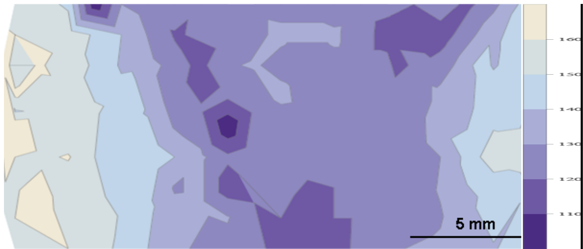
Figure 77. 10 mm Al 2024 FSW Hardness Mathematica Contour Plot. (171 Indents) Scale Indicates Vickers Hardness. Weld Regions are Represented by the Following Hardness Ranges: Weld Nugget from 110-130 Hv, TMAZ 140 Hv and HAZ 150-160 Hv
