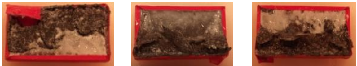
Figure 93. ASTM G34 Al 7075 Samples (a) Ground Substrate (b) Ground Substrate (c) As-Received Substrate
