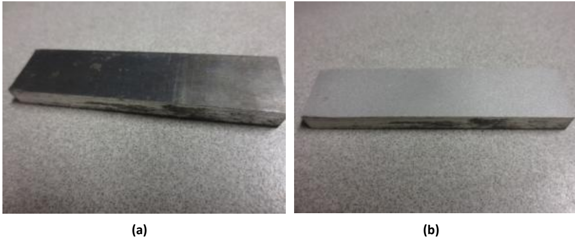
Figure 34. Bulk Al 7075 Coupon (a) Before and (b) After an 80 Grit Silicon Oxide Sand Blasting Process
