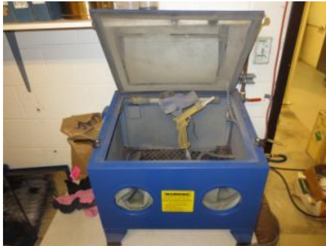
Figure 32. Dedicated Grit Blasting Chamber.
