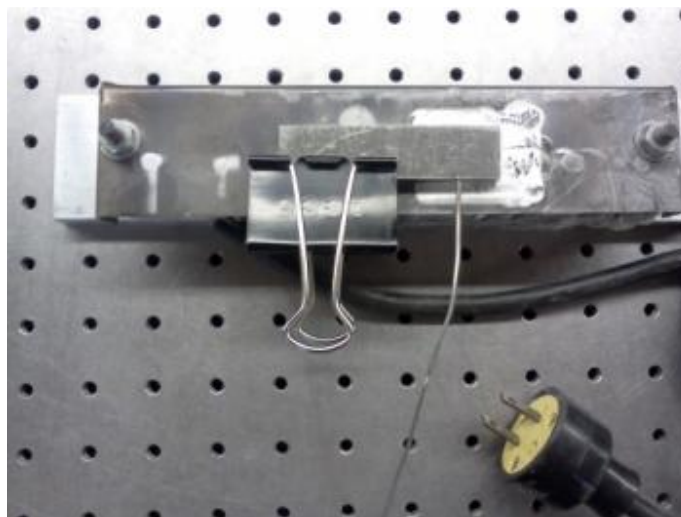
Figure 112. Heater Assembly with Substrate and Thermocouple Attached with a Paper Clip
