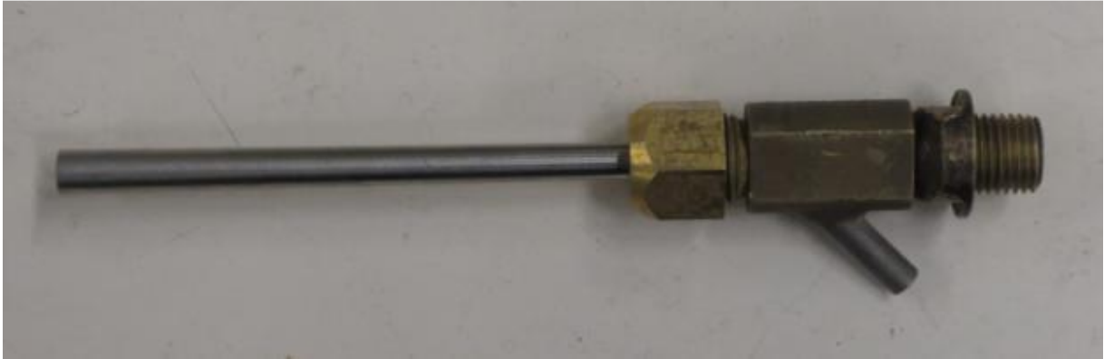
Figure 144. Assembled de Laval Metal Nozzle Assembly
