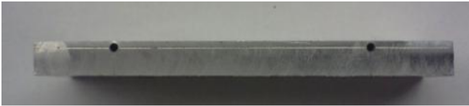
Figure 110. Side View of the Temperature Test Coupon with Thermocouple Entry Hole (Substrate is on Top Surface)
