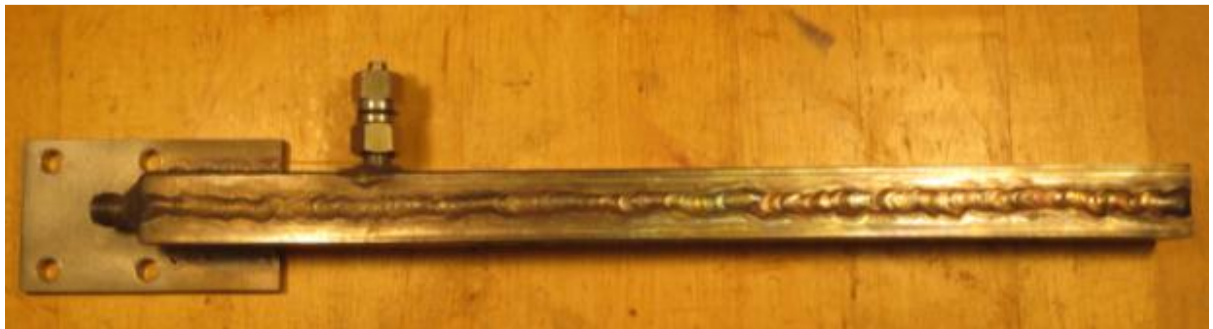
Figure 149. PR Nozzle. Propellant gas Inlet on the Left. Powder Injection on the Top.
