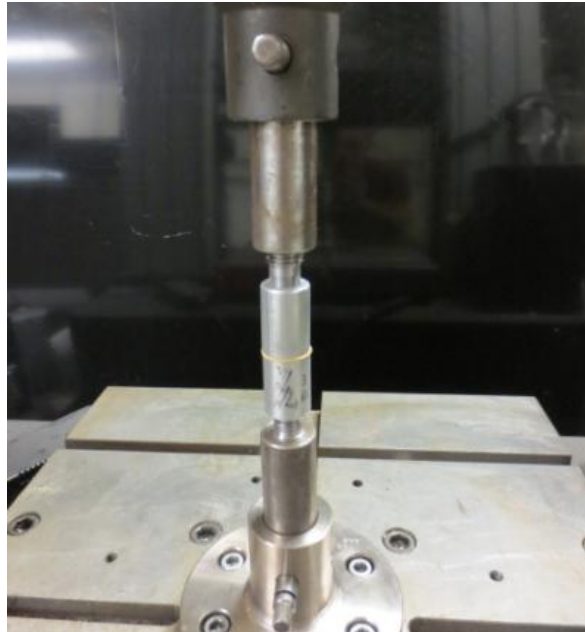
Figure 103. Tensile Specimen Mounted in a Universal Testing Machine, Ready for Testing
