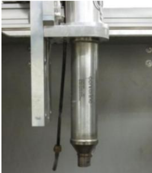
Figure 40. Propellant gas Heater. Within the Cabinet Assembly. Powder Feed Tube is Dangling Next to the Heater and Connects to the Nozzle Assembly Powder Inlet Tube
