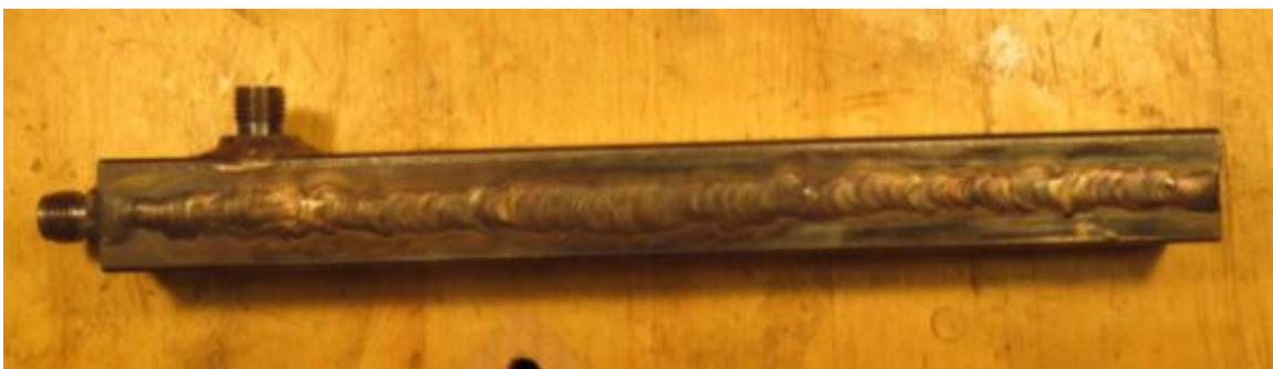
Figure 152. JM Nozzle General Side View. Propellant gas Inlet on Left, Powder Injection on Top.
