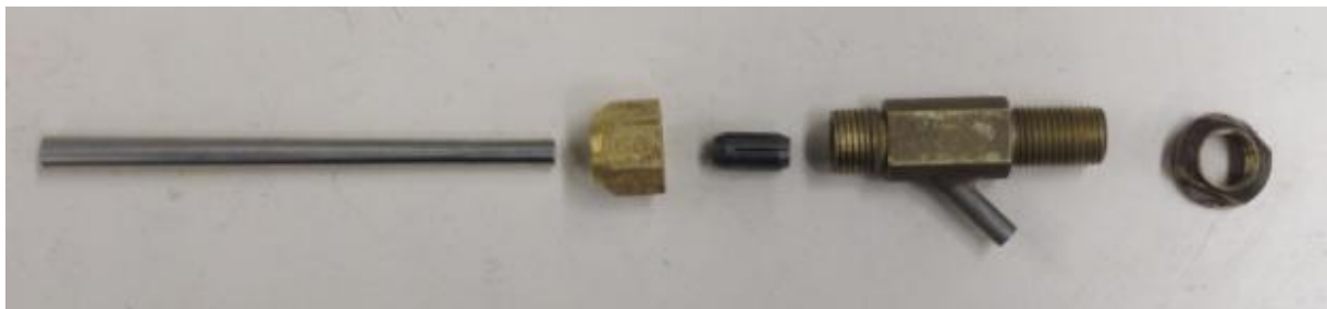
Figure 143. Disassembled de Laval Metal Nozzle Showing, From Left to Right, Stainless Steel Nozzle, Tightening Nut, Tightening Collet, Brass Orifice and Heater Nut
