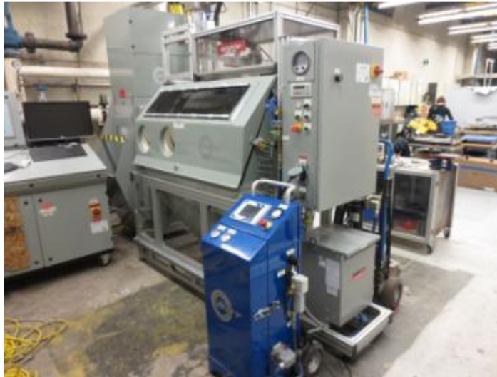
Figure 36. CGDS Equipment Overview
