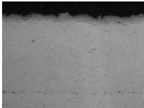
Figure 56. Example of a Fully Dense Al 7075 Coating, 100x, 590 \mu\text{m} Thickness
