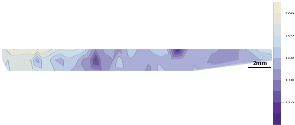
Figure 79. 2mm Al 7075 FSW Hardness Mathematica Contour Plot. (89 Indents) Scale Indicates Vickers Hardness. Weld Regions are Represented by the Following Hardness Ranges: Weld nugget 120 – 140 Hv, TMAZ 150-160 Hv and HAZ 170-200 Hv
