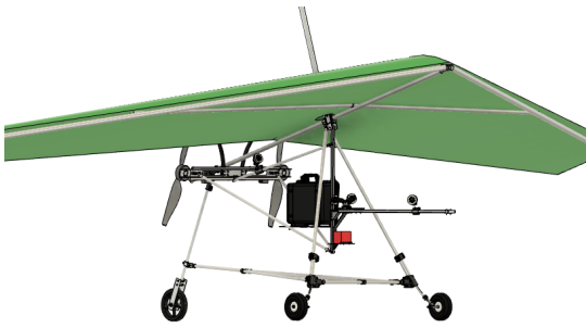
Fig. 2. 3D computer-aided design model of the Romaeris uncrewed weight-shift aircraft prototype.
