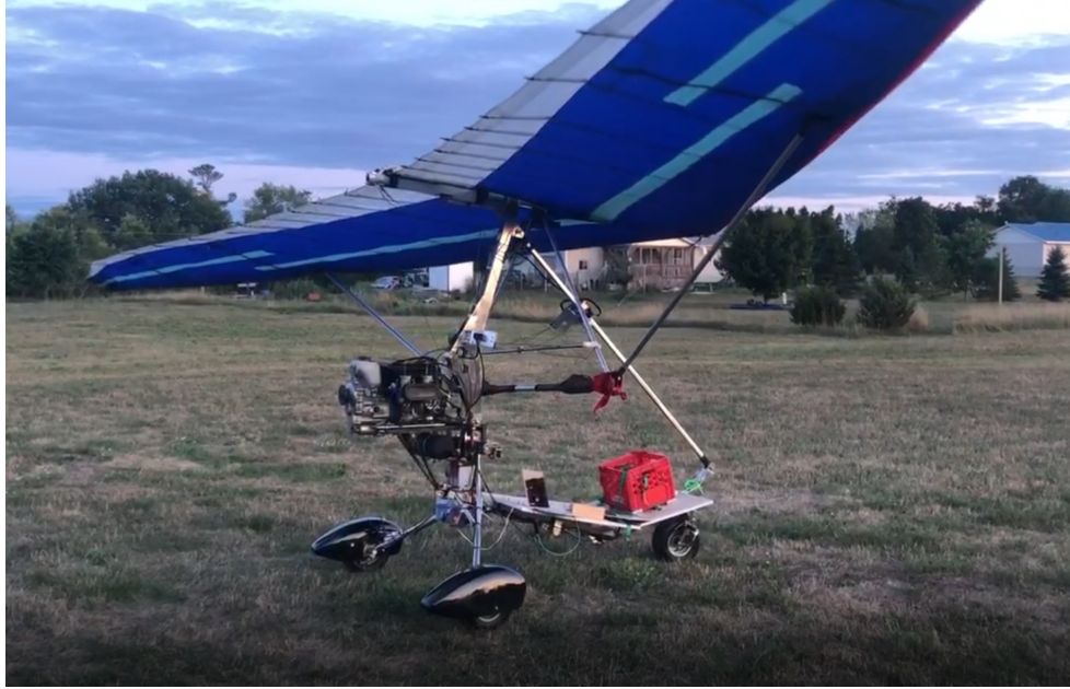
Figure 1.1: A prototype unmanned weight-shift control aircraft, with a cable-driven parallel manipulator system attached. WSC aircraft consist of two main bodies: the wing and the fuselage.
