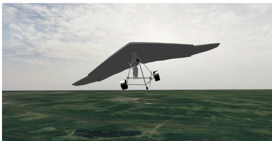
Fig. 1. Capture from Gazebo simulator of the uWSC aircraft model performing a starboard side banking turn. The hung mass under the wing is responsible for attitude adjustments via weight-shifting control.
