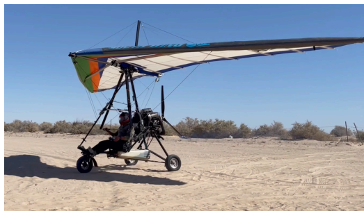
(a) Experimental weight-shift aircraft.
