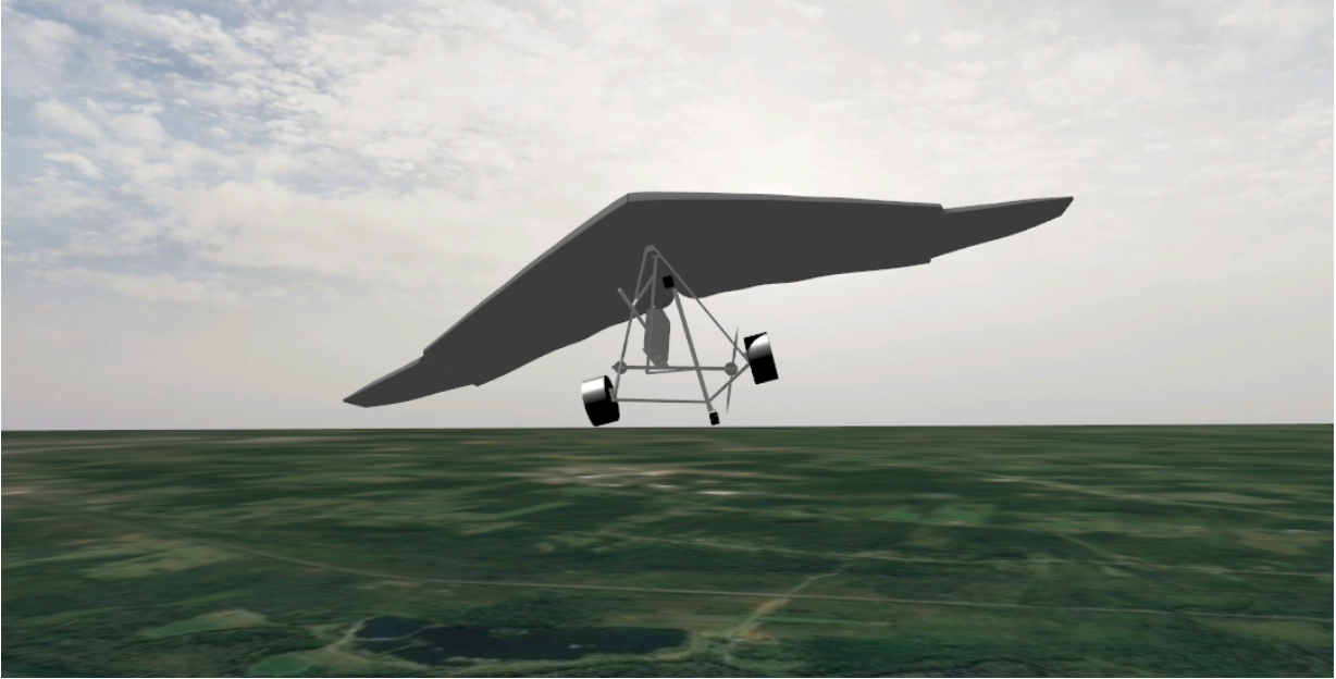
Figure 5.1: Capture from Gazebo simulator of the uWSC aircraft model performing a starboard side banking turn. The hung mass under the wing is responsible for attitude adjustments via weight-shifting control.
