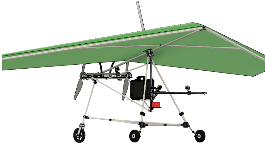
Figure 5.2: 3D CAD model of the Romaeris uncrewed weight-shift aircraft prototype.
