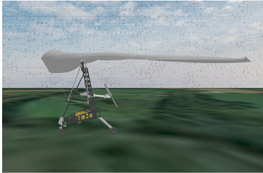
(a) Gazebo model for the prototype unmanned weight-shift aircraft.
