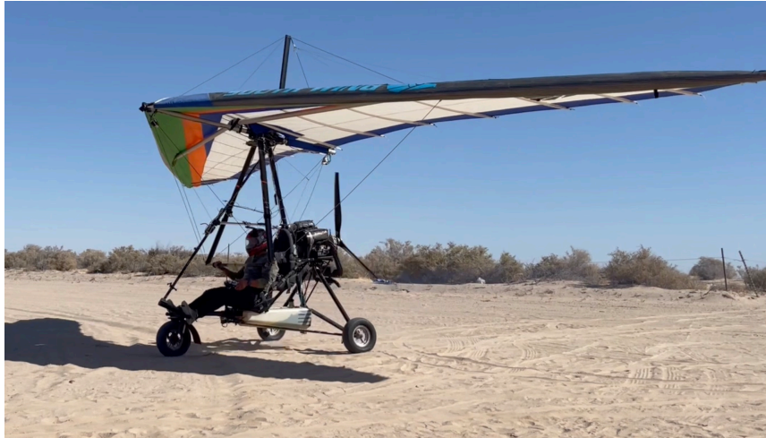
(a) Experimental weight-shift aircraft.
