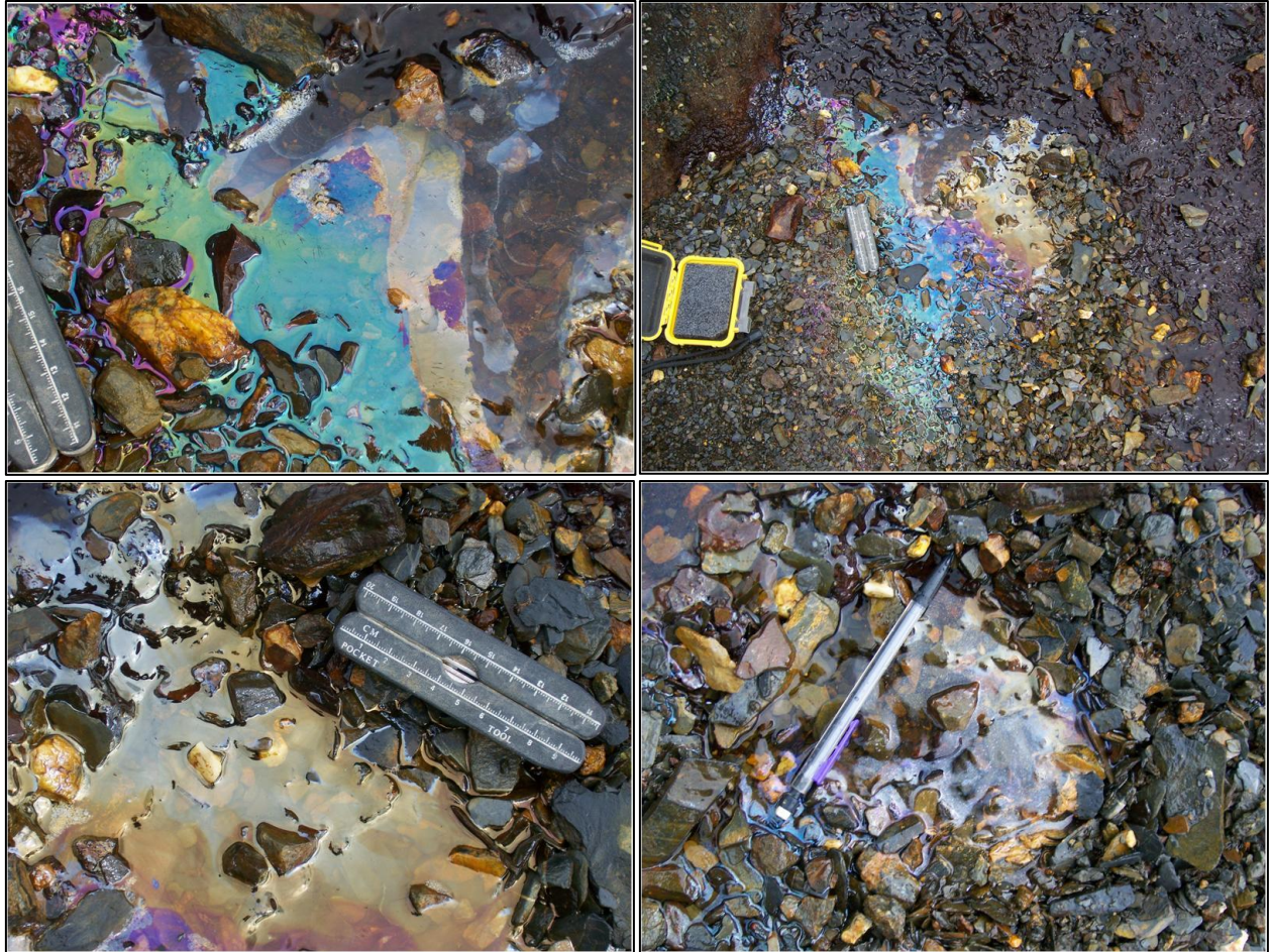
Figure 23: Thin, sheeny films found in areas near the groundwater seeps and in the upper reaches of the creek near the end of the sampling campaign. Sheeny appearance may be due to the presence of waste products from Fe-oxidizing bacteria.
