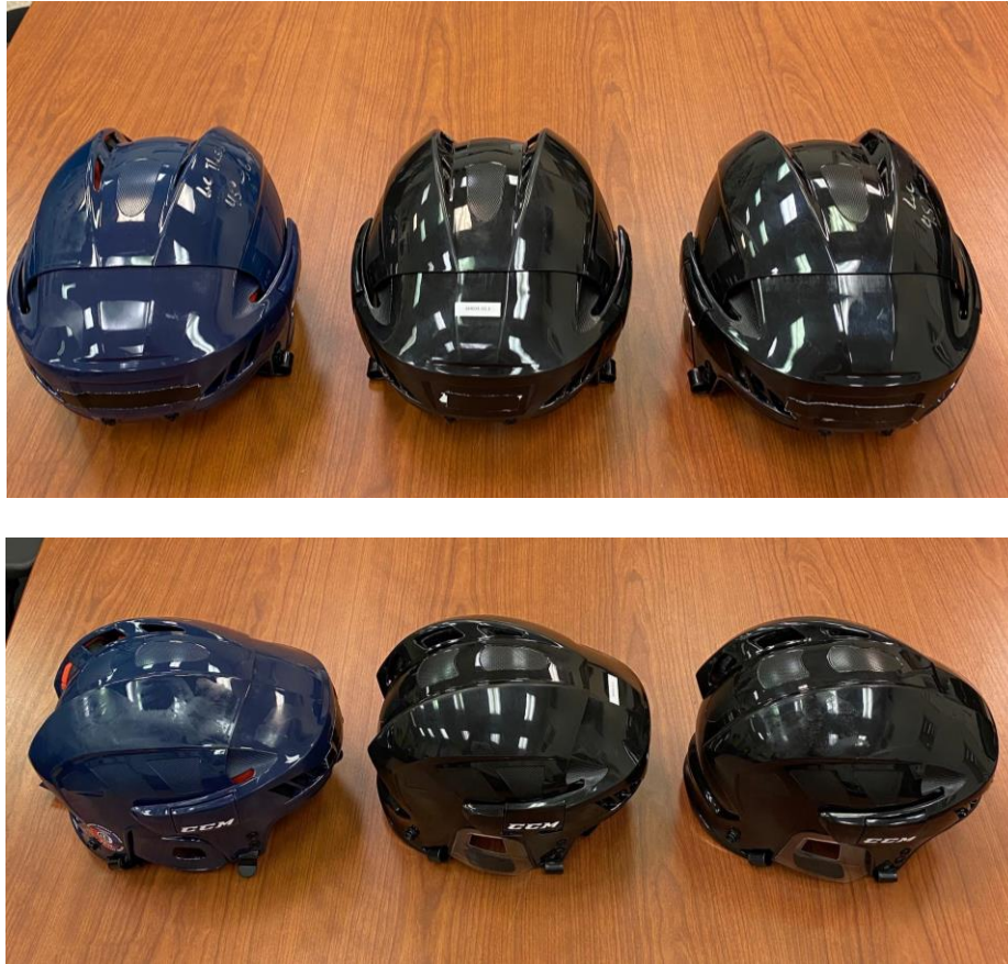
Figure 5. Front and side view of the helmet shells for the 50 (left), XT99 (middle), and Prototype (right) helmets
