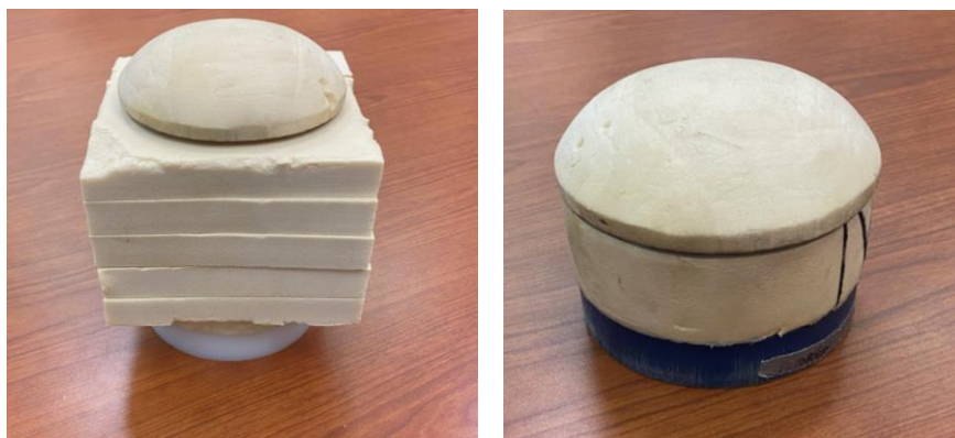
Figure 2. The high (left) and medium (right) compliance impactor caps with 25 and 15 ms durations, respectively.
