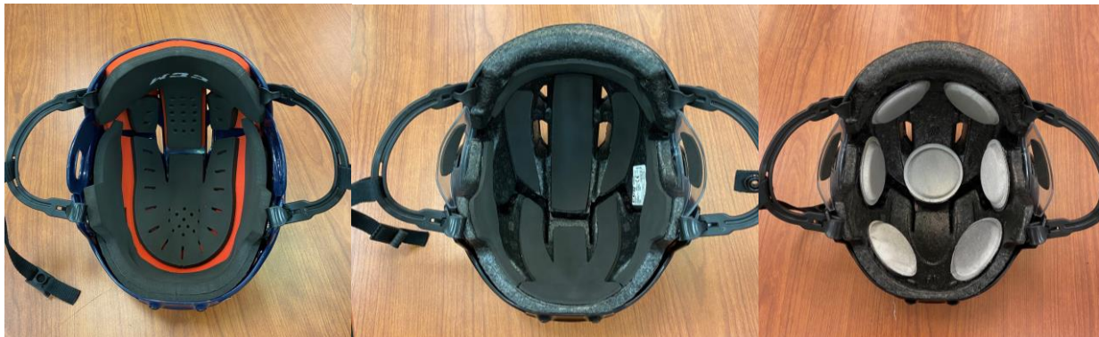
Figure 4. CCM 50 helmet with VN foam (left, CCM XT99 helmet with EPP liner with comfort foam (middle), prototype helmet using the XT99 helmet with oil filled pods (right).
