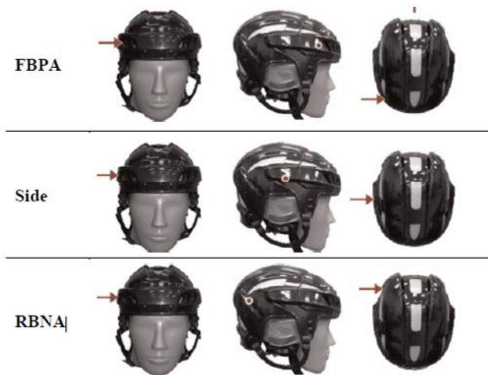
Figure 3. Impact locations for the pneumatic ram tests viewed in the sagittal, frontal, and transverse planes with the impact vectors indicated by the arrows.
