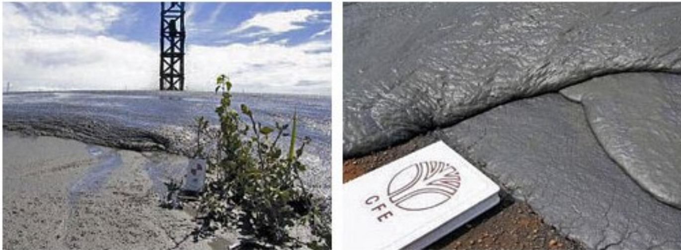
Figure 2.14. Deposition of fresh paste tailings layers at the Bulyanhulu gold mine in Tanzania (Engels, 2002; Theriault et al., 2003)
