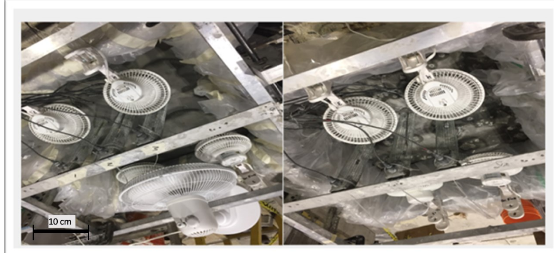
Figure 5.5. Pictures of the commercial fans used to dry the tested tailings
