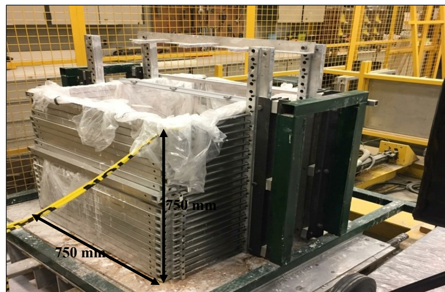
Figure 6.6. Photo of the flexible laminar shear box (FLSB) used in this research
