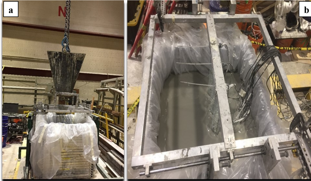
Figure 4.5. (a) Snapshot showing the concrete bucket that was used for deposition of thickened tailings layers. (b) Snapshot of the ground surface of thickened tailings shortly after deposition of the third (top) layer
