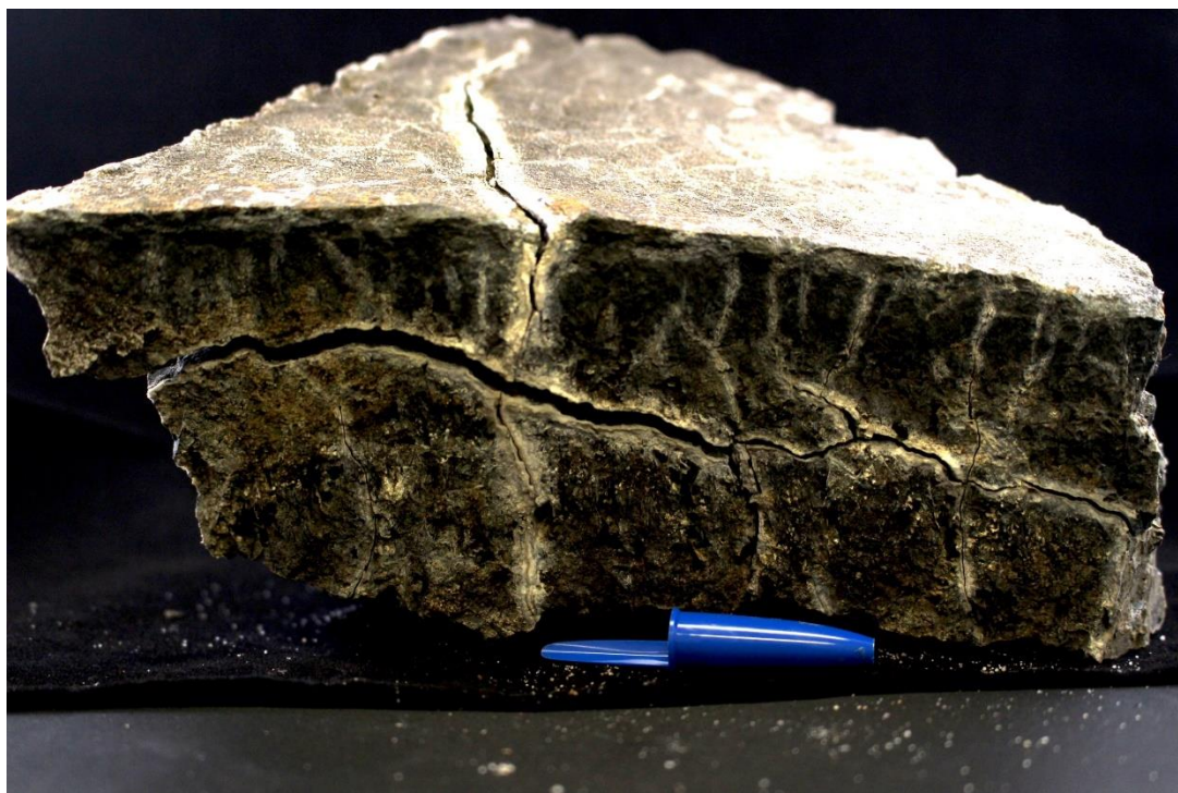
Figure 3. Oka slag with white alteration product accumulated around cracks
