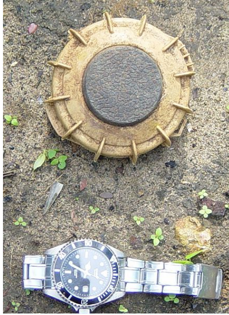
Figure 1.2: A VS-50 landmine next to a wrist watch. Despite being very small it can generate a shock wave strong enough to produce a TBI. Picture taken by Clark [2].
