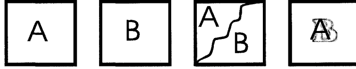
Figure 6.2: Four cases in a combinative fusion. For a small local region in the fused image, the local feature may come from the corresponding block of the input image A or B, or a combination of them.
