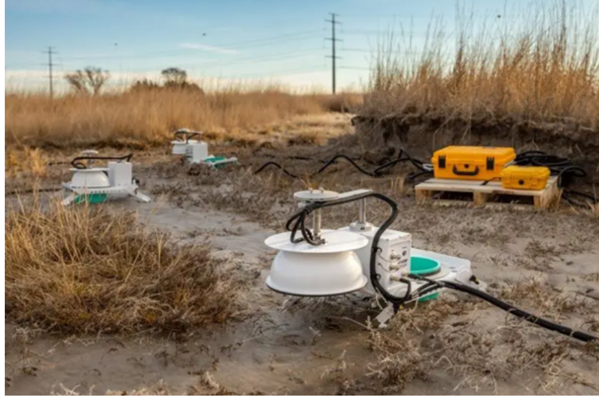
Figure 3.3: LI-COR sensor. LI-COR Gas Analyzers are high-precision instruments used for measuring greenhouse gas (GHG) fluxes, including nitrous oxide ( \text{N}_2\text{O} ), methane ( \text{CH}_4 ), and carbon dioxide ( \text{CO}_2 ), from soil, water, and air. These sensors can detect gas concentrations with high accuracy. In agricultural and environmental research, LI-COR chambers are commonly deployed to capture real-time \text{N}_2\text{O} emissions from soil, providing direct, empirical measurements that are essential for validating predictive models. These sensors are widely used due to their high sensitivity and ability to operate in field conditions. However, this technology is costly. Image and description from LI-COR Environmental (2026).
