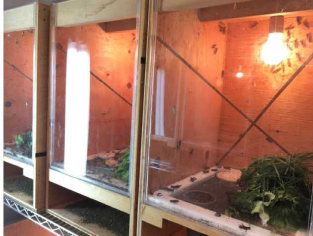
Figure C.1 Melanoplus sanguinipes colony rearing cages. Each wooden cage is fitted with a Plexiglass front, insect screening floor, a 40-watt incandescent lightbulb for warmth and perches for grasshoppers.
