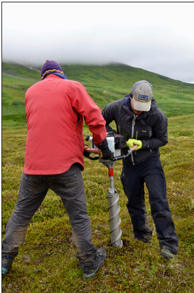
Figure 17: Core drilling within the hummock top with the CREEL at field 12 (N 59.67565° W 136.68051°)
