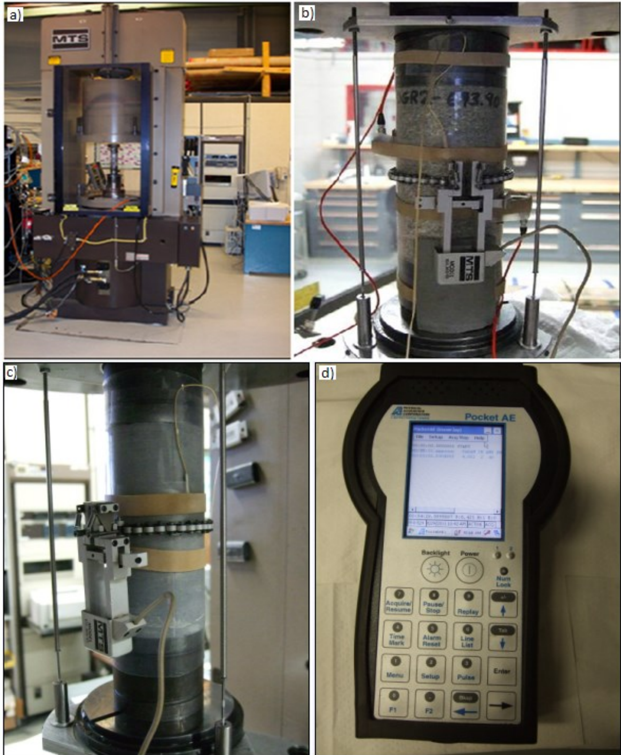
Figure 4.5: Testing equipments: a) MTS Rock Mechanics Testing System, b) setup using a granite specimen, c) setup using Tournemire argillite specimen, and d) Acoustic emission device.
