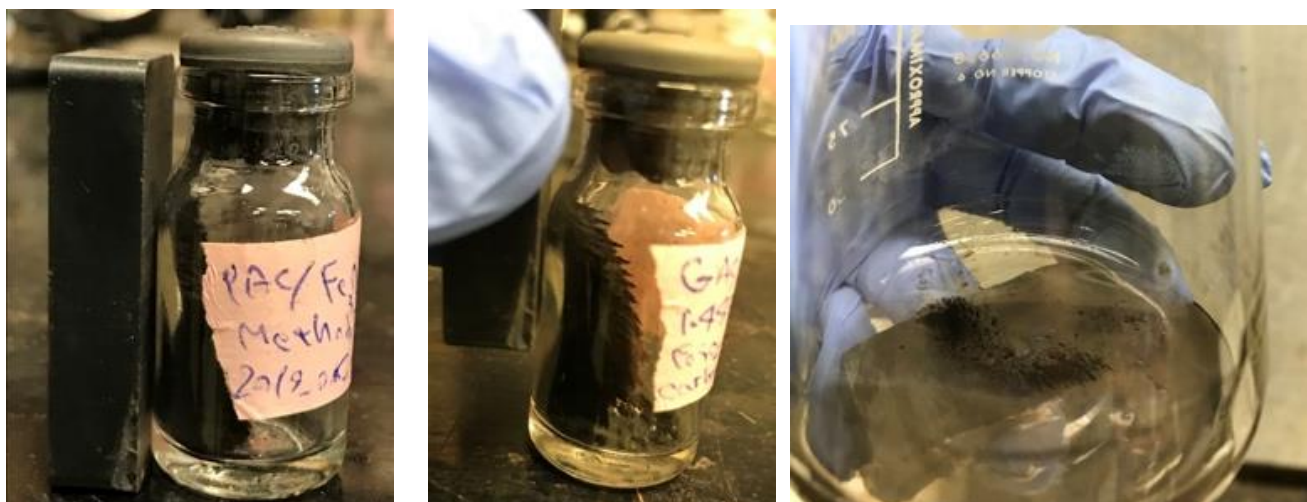
Figure 2.2. Recoverable AC/Fe 3 O 4 particles with high surface area and superparamagnetic characteristics
