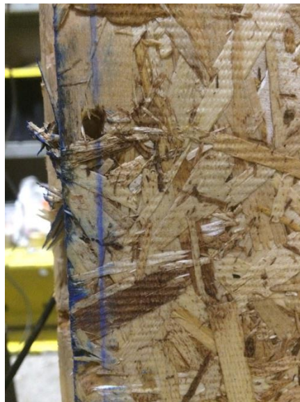
Figure 5.17: Nails Pull-Through (Nail End/Edge Distance: 9.5mm)
