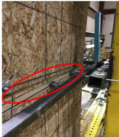
a) Yielding of Nails, Nails Pull-Through
