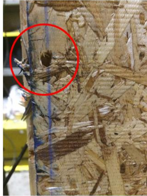
b) SW-4D Nails Pull-Through
