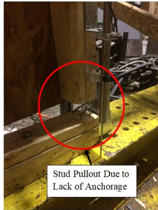
c) Stud Pullout at Tension Side
