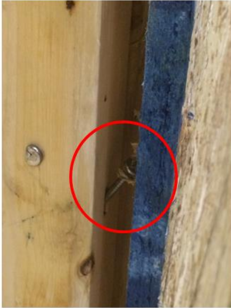
a) SW-4A Nails Yielding, Nails Pull-Through
