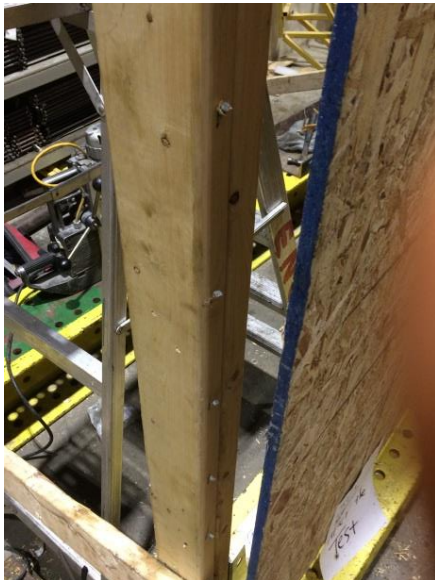
a) SW-1A-R2 Nails Yielding, Nails Pull-Through
