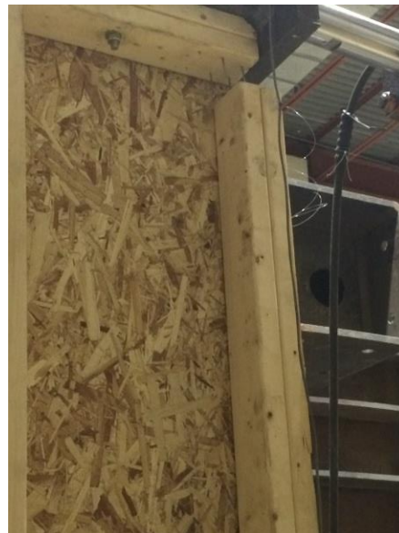
b) SW-1A-R2 Nails Withdrawal at Top Plate
