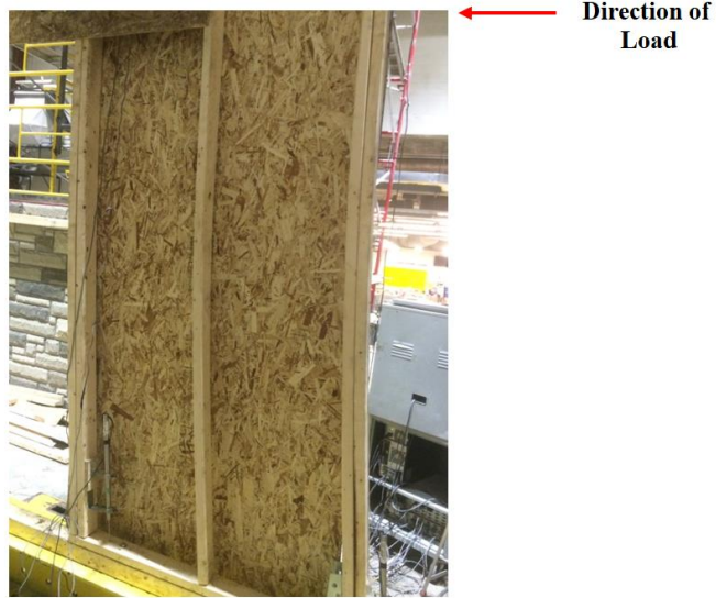
Figure 4.9: SW-2I Studs Bending
