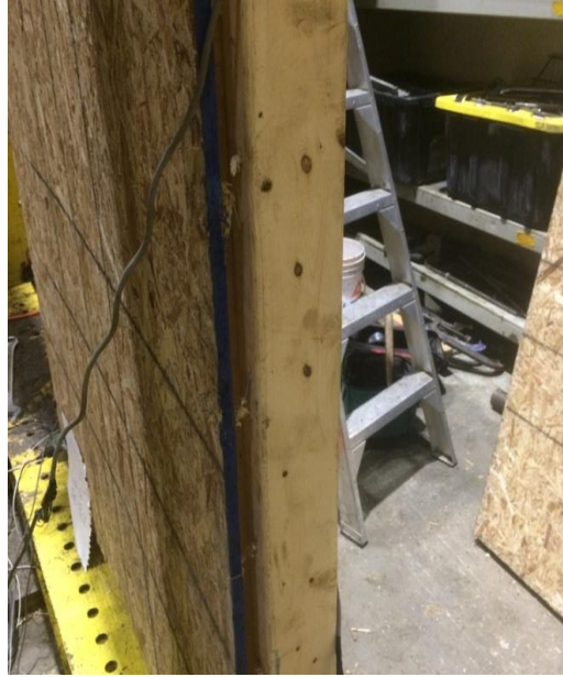
Figure 4.13: SW-5B Uniformly Distributed Yielding of Nails through the Entire Wall Followed by Nails Pull-Through Towards End of the Test
