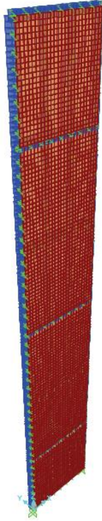
Figure 6.9: 3-D View of 6-Storey Shear Wall Assembly
