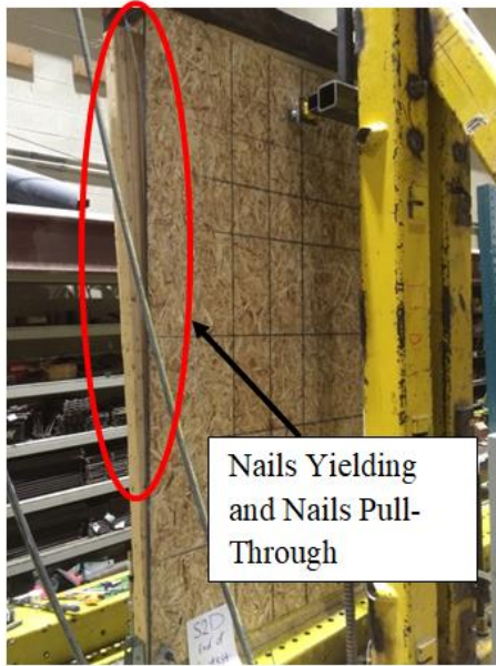
a) SW-2B Nails Yielding, Nails Pull-Through
