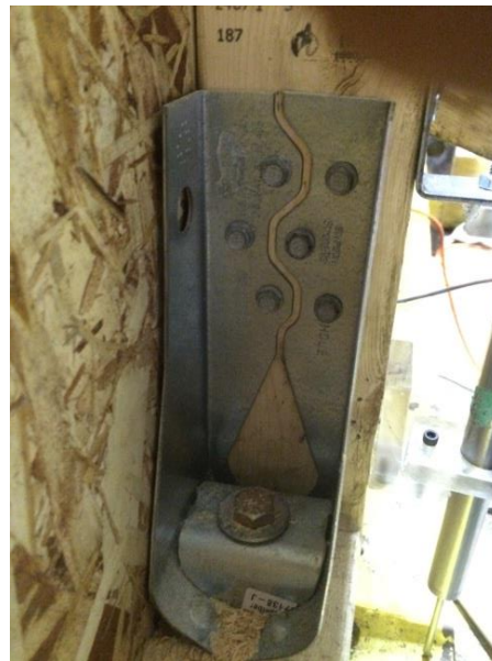
Figure 3.2: HDU2 Hold-Down Installation
