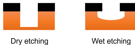
FIGURE 1.21: Schematic representation of dry- and wet-etching processes.
