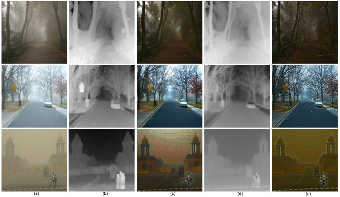
Figure 3.10: (a) Input foggy images. (b) Estimated depth map by He et al. [89]. (c) Restored images using (b). (d) Estimated depth map by our work, (e) Restored images using (d).
