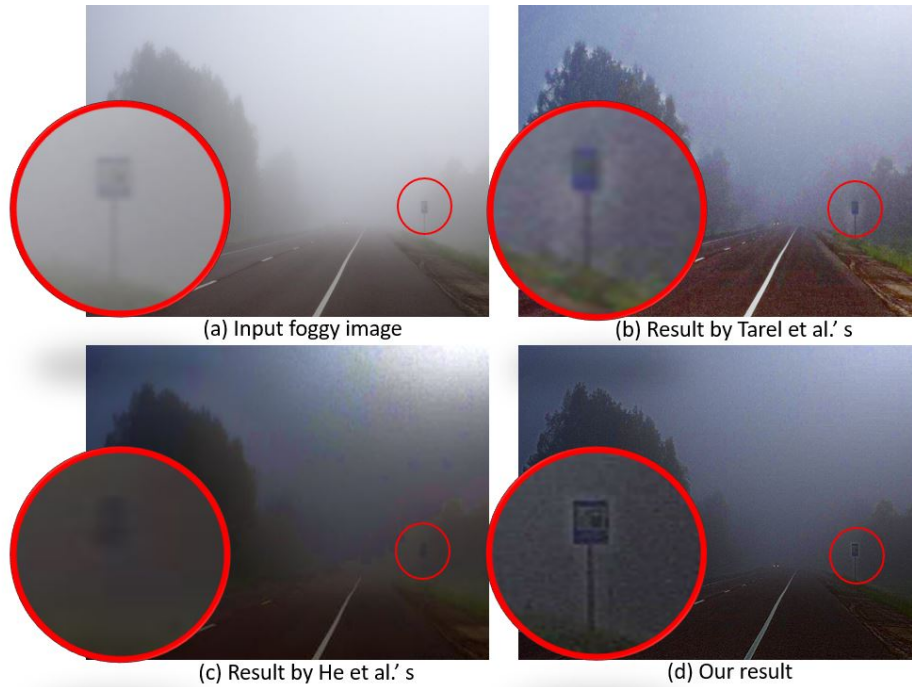
Figure 4.11: Comparisons of the visibility of traffic signs after restoration by some defogging algorithms on real images. (a) Input foggy image. (b) Tarel and Hautiere [176]. (c) He et al. [89]. (d) our result.
