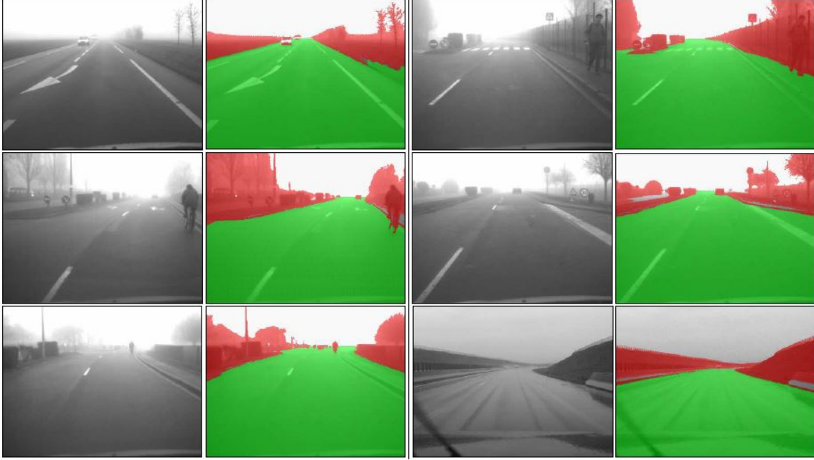
Figure 2.6: First and third columns are original foggy images. Second and fourth columns are the results of vertical objects segmentation and road plain area which can be seen as red and green colors, respectively [85].
