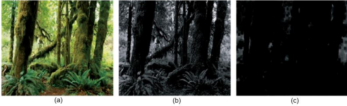
Figure 3.8: Estimation of a dark channel. (a) An arbitrary image B . (b) Calculation of minimum value of each pixel. (c) A minimum filter is performed on (b). This is the dark channel of B . The patch size of \Omega is 15 \times 15 [89].
